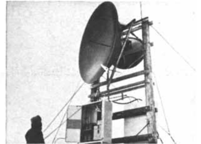
Merrimack Valley Laboratory, Mass. We were increasing the capabilities of a new microwave system designed for low-cost telephone and television communications over distances up to 200 miles. This system is based on advances in solid state technology.
