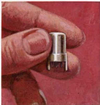
RCA NUVISTOR TUBES combine highly effective performance with extremely small size and light weight.
