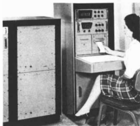
This data system, incorporating a digital voltmeter and other standard instruments, measures and records up to 300 widely varying temperatures.
