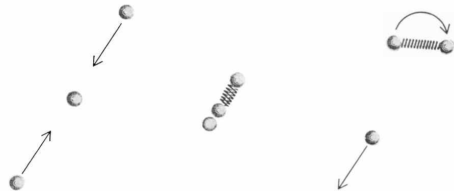
THREE-BODY RECOMBINATION is the reverse of the dissociation process shown in the illustration above. Two particles form an interatomic bond in a collision with a third particle. The third particle leaves the collision with more energy than it had originally.
