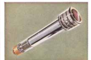
RCA Image Orthicon Tube is the all-seeing "eye" of the TV Camera.
