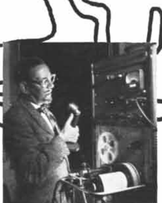
Word Picture. This is a picture of the spoken word "you." By analyzing the sound with a spectrograph, the Laboratories' Lawrence G. Kersta makes a print of the word in graph form. Graph shows frequency, time taken, and intensity used in making speech sound.
