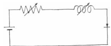
Diagram of tunnel diode oscillator
