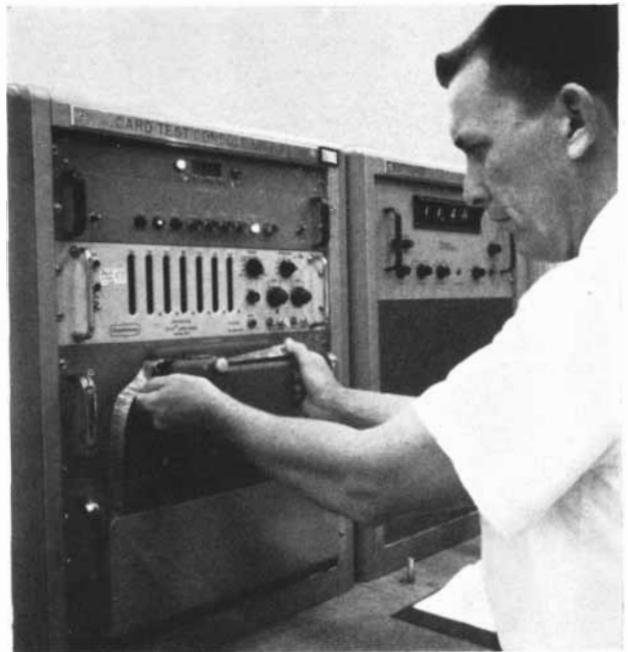
Carle W. Collins, production test engineer, Martin Company's Orlando (Fla.) Division, inserts coded Mylar tape into the reader unit of the Tape Programmed Automatic Tester which he designed.
