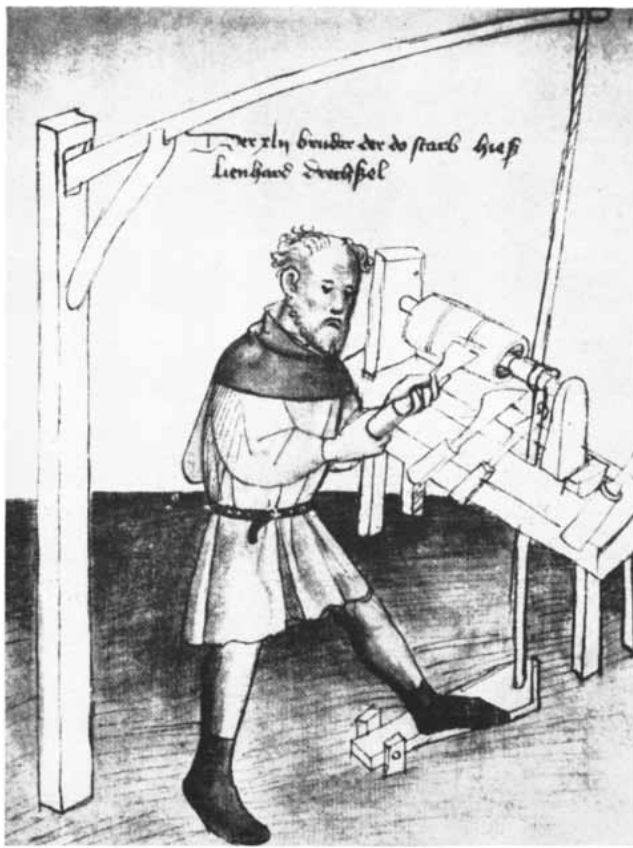
POLE LATHE OF 1395 enabled the workman to turn the workpiece by means of a foot treadle and freed both of his hands for holding the cutting tool. The workpiece rotated back and forth.
