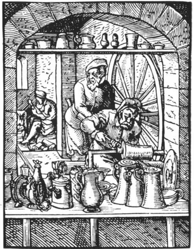
CONTINUOUS-DRIVE LATHE OF 1568 eliminated the back-and-forth rotation of the workpiece, produced by pole-and-treadle lathe, but required the services of a helper to turn a drive wheel.
