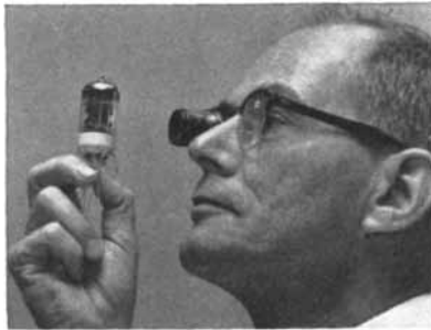
Allentown Laboratory, Pa. We were working with engineers of Western Electric, manufacturing unit of the Bell System, on the manufacture of long-life electron tubes for a new deep sea cable system.
