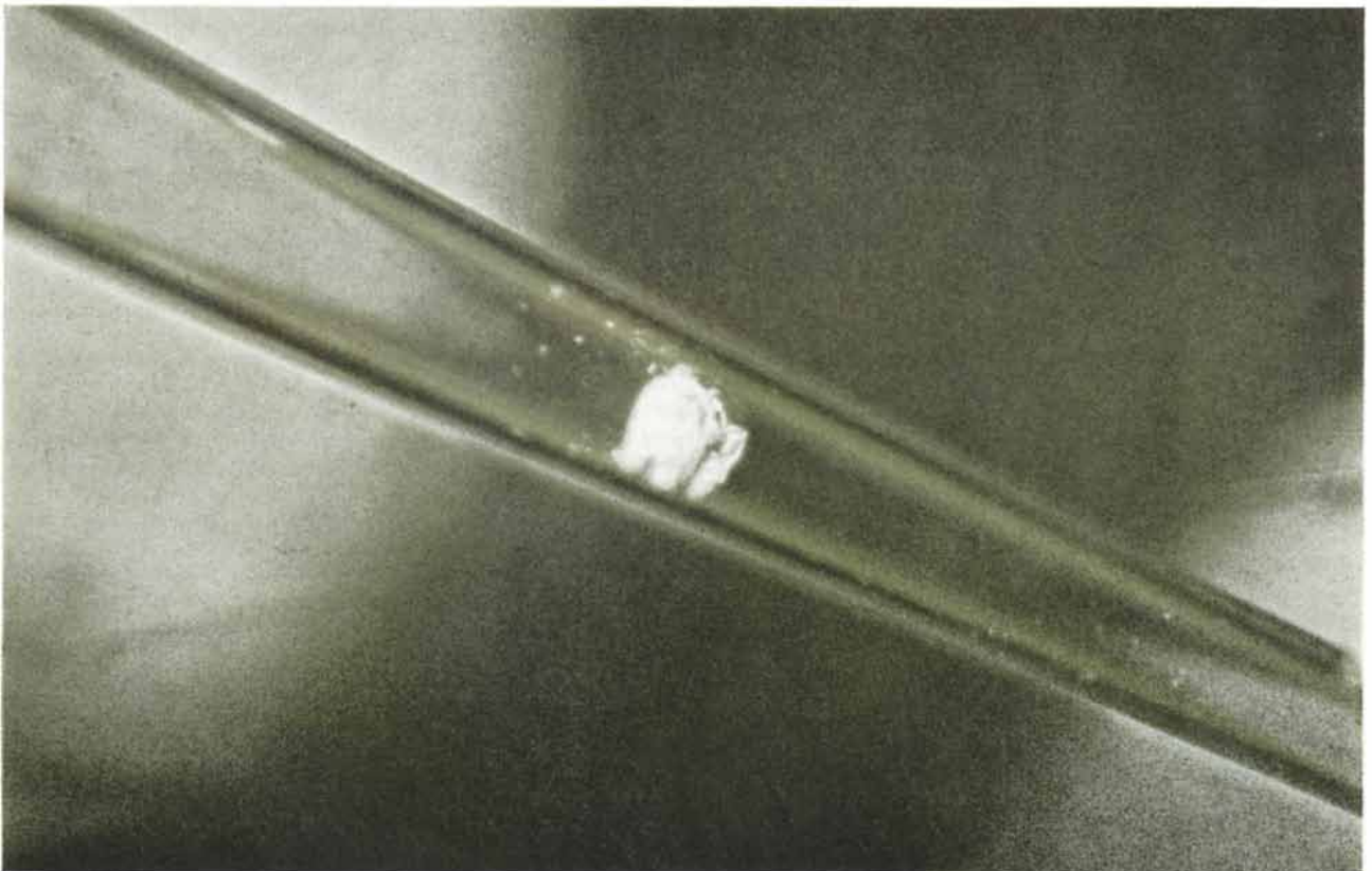
CALIFORNIUM , element 98, discovered in 1950, was obtained in a compound in visible quantity in 1960. The speck of californium
