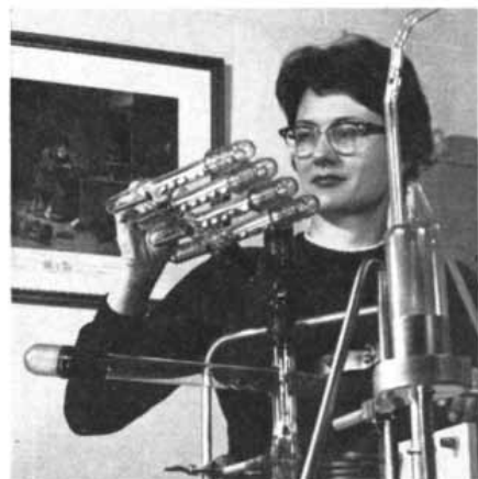
Anaconda research chemist Virginia Horigan manipulates copper samples to release captive oxygen and hydrogen atoms for measurement of low level gas content of copper alloys.
