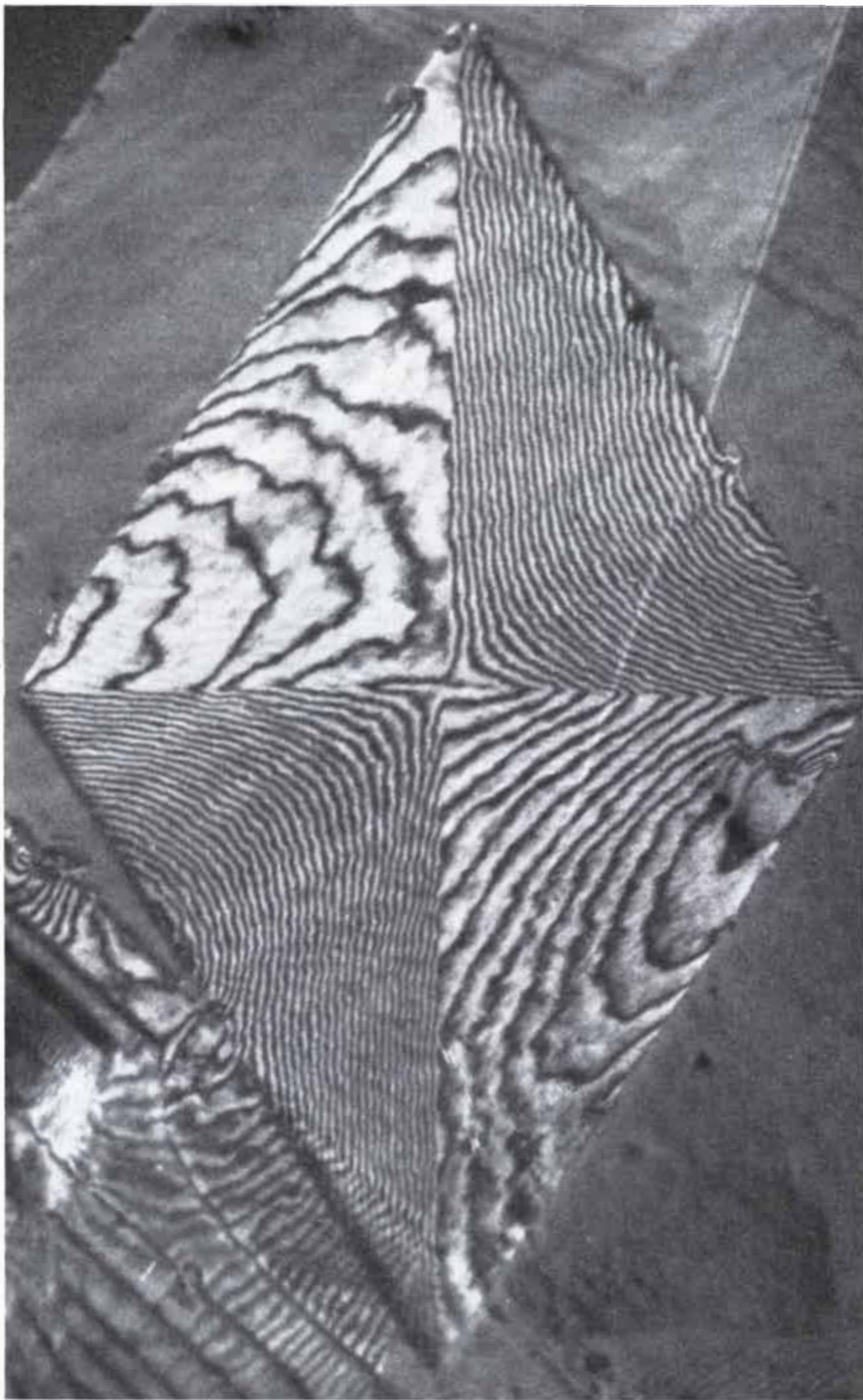
MOIRÉ CREATED BY TWO CRYSTALS appears in this remarkable electron micrograph made by V. F. Holland of the Chemstrand Research Center, Inc., in Durham, N.C. The picture shows a crystal of polyethylene grown on a layer crystal of the same polymer. The moiré appears because the atomic lattices of the two crystals happen to be in almost direct alignment; the closer the alignment, the wider the spacing between the moiré fringes.
