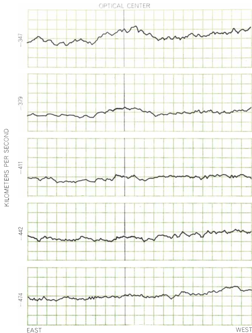
MULTICHANNEL DRIFT CURVES of irregular galaxy IC 10 were obtained in one sweep with maser mounted on the 60-foot telescope of Harvard College Observatory. Different frequencies recorded represent velocity differences of about 30 kilometers per second. Responses here show that this galaxy is receding at approximately 347 kilometers per second.
