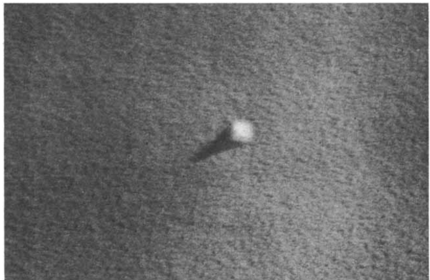
MESOPAUSE PARTICLES such as this one, collected during rocket flight into sky empty of noctilucent clouds, produced no halo on aluminum or dye surfaces. Collecting surfaces from cloudless mesopause contained 100 to 1,000 fewer particles than those flown into cloud.
