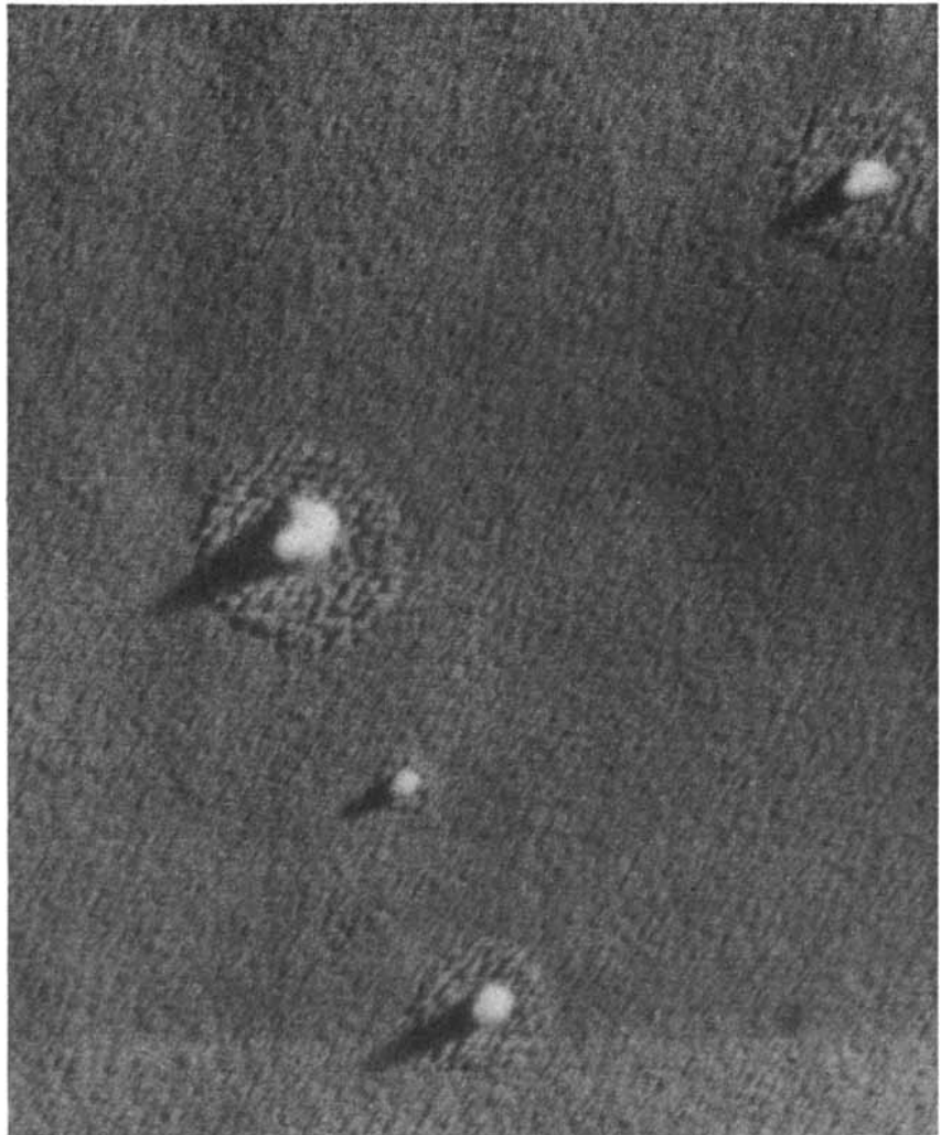
NOCTILUCENT CLOUD PARTICLES were captured on an aluminum-nitrocellulose surface during rocket flight. Particles are nonvolatile, but many are surrounded by halos presumably made by volatile material. The particles are enlarged about 30,000 diameters in this electron micrograph, which was made at Air Force Cambridge Research Laboratories.
