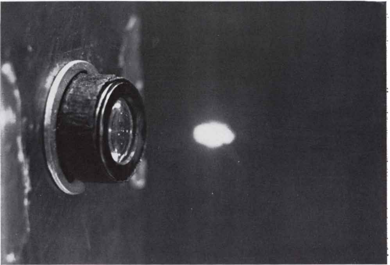
ELECTRICAL BREAKDOWN OF AIR is produced by the focused beam of a giant-pulse ruby laser. Such lasers incorporate a shutter to postpone stimulated emission, thereby raising beam intensity.
