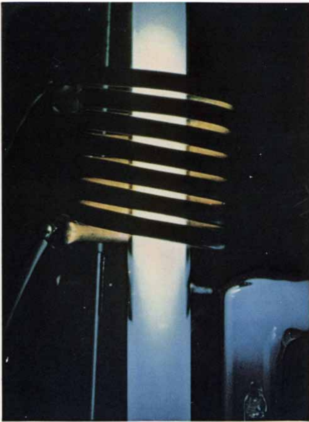
Vapor of carbon tetrachloride ionized by high-frequency field
