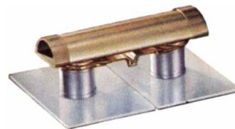
Segment of thermoelectric module used in electric power generation (shown approximately one-half actual size).
