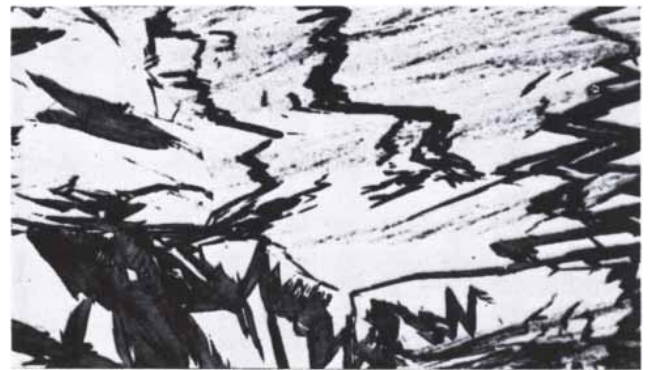
MARTENSITE PLATES , dark jagged shapes, grow to large size ( lower left ) in nondeformed region of martensite. In deformed region ( upper right ) plates are deflected when they meet slip bands.
