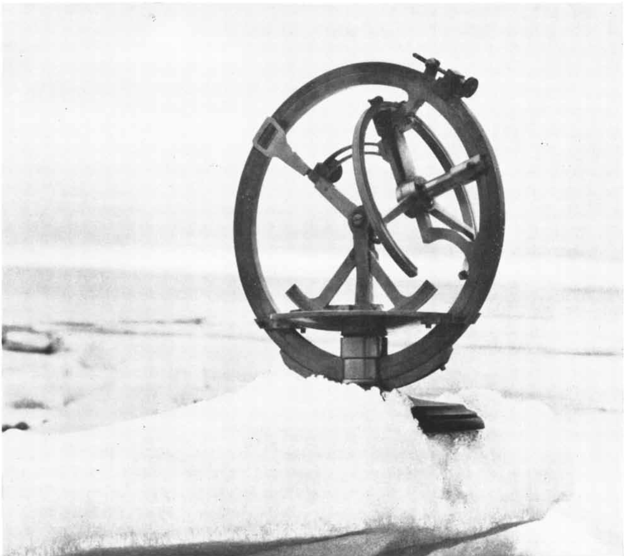
Solar Compass (American-1836)—Used to indicate the direction of true north by a single observation of the sun's position. A similar device was used in 1926 by Adm. Richard E. Byrd on his historic flight over the South Pole, an area where anomalies render the magnetic compass inaccurate. (Dossin Museum)
