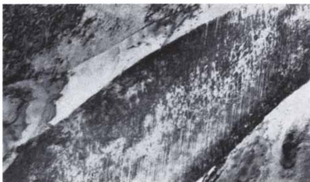
TWINNED MARTENSITE PLATES appear as fine parallel lines in this electron micrograph of Ausform steel by P. M. Kelly, University of Leeds. Such crystal twins block movement of dislocations.
