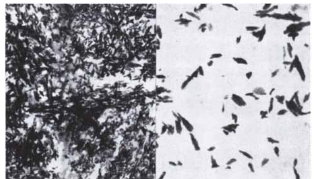
CARBIDE PARTICLES larger than 50 angstrom units in size are shown in ordinary martensitic steel ( left ) and in Ausform steel ( right ). Most Ausform carbon is in solution or in fine particles.
