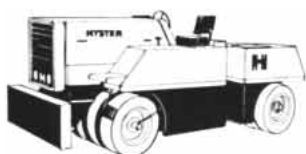
C500A Pneumatic Compactor, one of five types of Hyster earth compaction machines.
