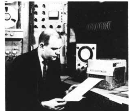
The Honeywell reproducing and amplifying tape system and the Model 906 Visicorder Oscillograph in Lessells' Boston laboratory.
