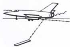
West Germany: A Bliss arresting gear "catches" a landing U. S. A. F. jet fighter on the runway after a brake failure.
