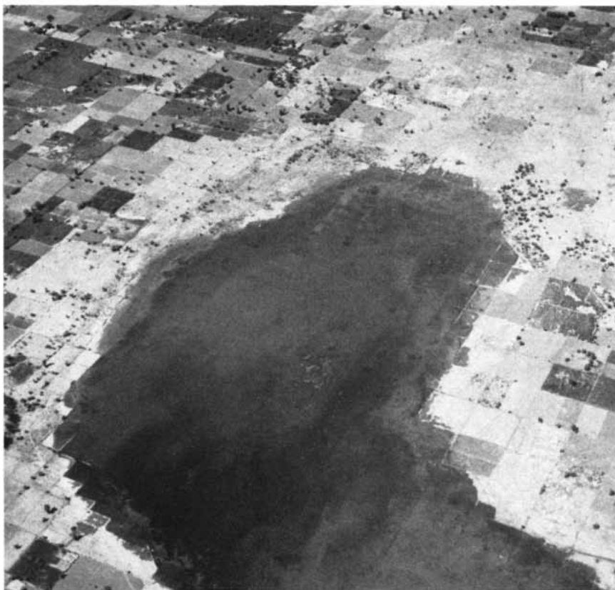
WATERLOGGED FIELDS near Sargodha in Pakistan reflect leaky canal system and inadequate drainage. Cultivated plots can be seen under water in center of photograph. When it evaporates, the water will deter renewed cultivation by leaving salts in topsoil.
