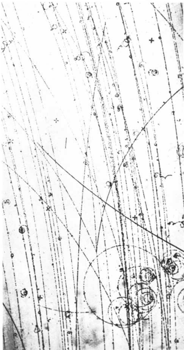
DECAY IN FLIGHT of K-minus particle is shown in bubble-chamber photograph made at the Brookhaven National Laboratory and in the accompanying map at right. The track of the K-minus
