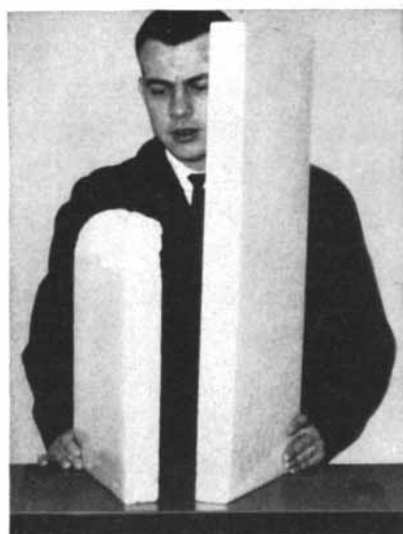
Rigid urethane foam (right) with silicone surfactant added.
