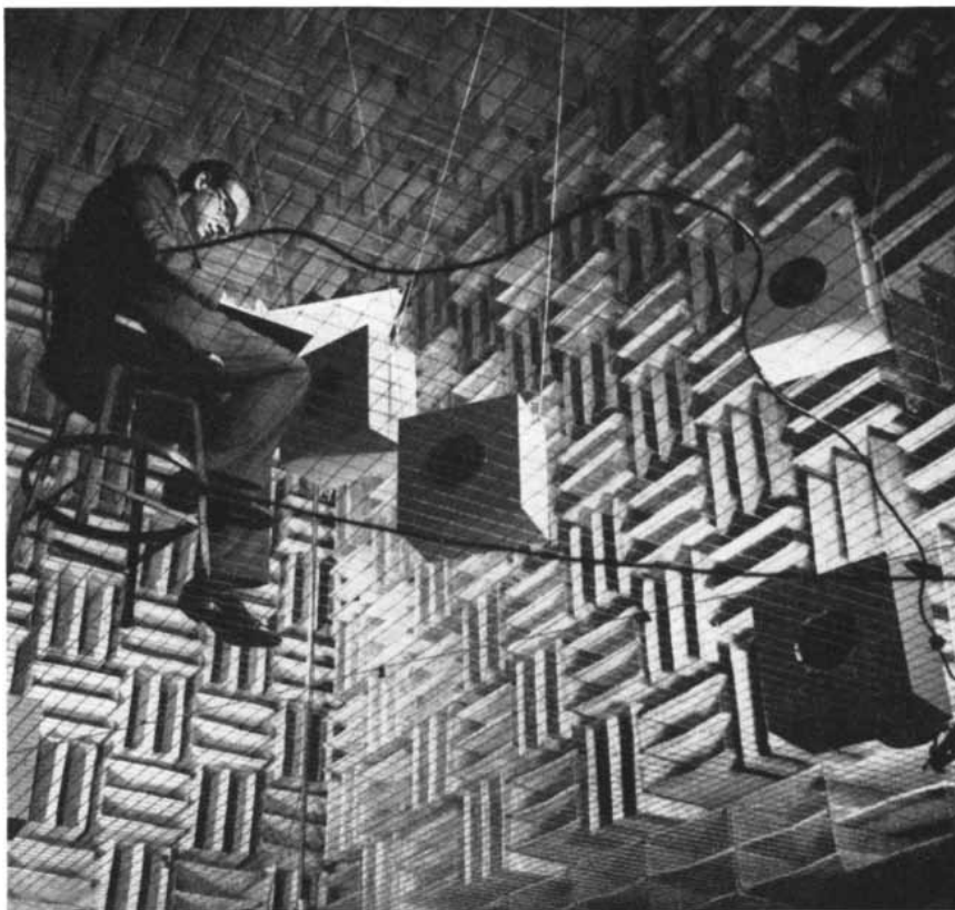
ANECHOIC CHAMBER is employed by Manfred R. Schroeder of Bell Telephone Laboratories to evaluate stereophonic playback of a sound recording that has been modified by a computer to simulate the acoustics of a newly designed music room or concert hall.
