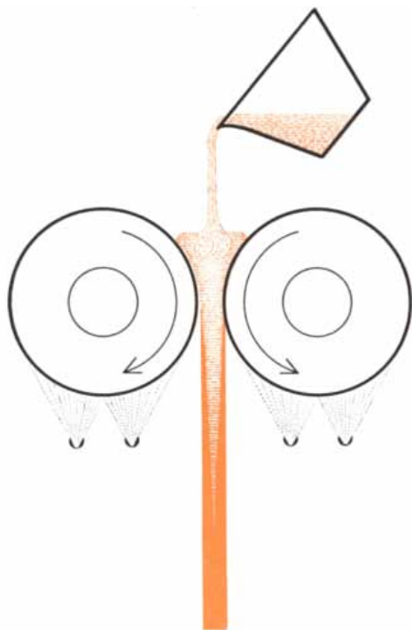
BESSEMER PATENT granted in 1865 called for pouring metal between two water-cooled rollers to form a solidified plate.
