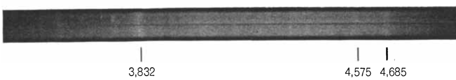
SPECTROGRAMS OF 3C 48, made by the author, show three weak emission lines at 3,832, 4,575 and 4,685 angstroms. The illustration actually consists of two spectrograms placed side by side to increase the visibility of faint lines. Even so, the three lines labeled are almost submerged by the continuum radiation of the object. Also visible are a number of prominent night-sky lines produced by air glow in the upper atmosphere. Close inspection of these and other spectrograms disclosed three more very faint emission lines at 4,066, 5,098 and 5,289 angstroms. The six emission lines were identified by assuming that their rest wavelengths had been red-shifted approximately 37 per cent, as illustrated on the opposite page.
