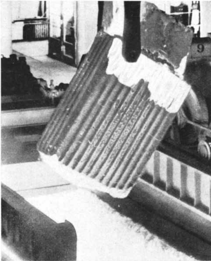
SOAKING PIT at the Bethlehem plant in Johnstown, Pa., receives an ingot from an overhead crane. Before rolling, the ingot is reheated in the gas-fired furnace to a uniform 2,200 degrees Fahrenheit.
