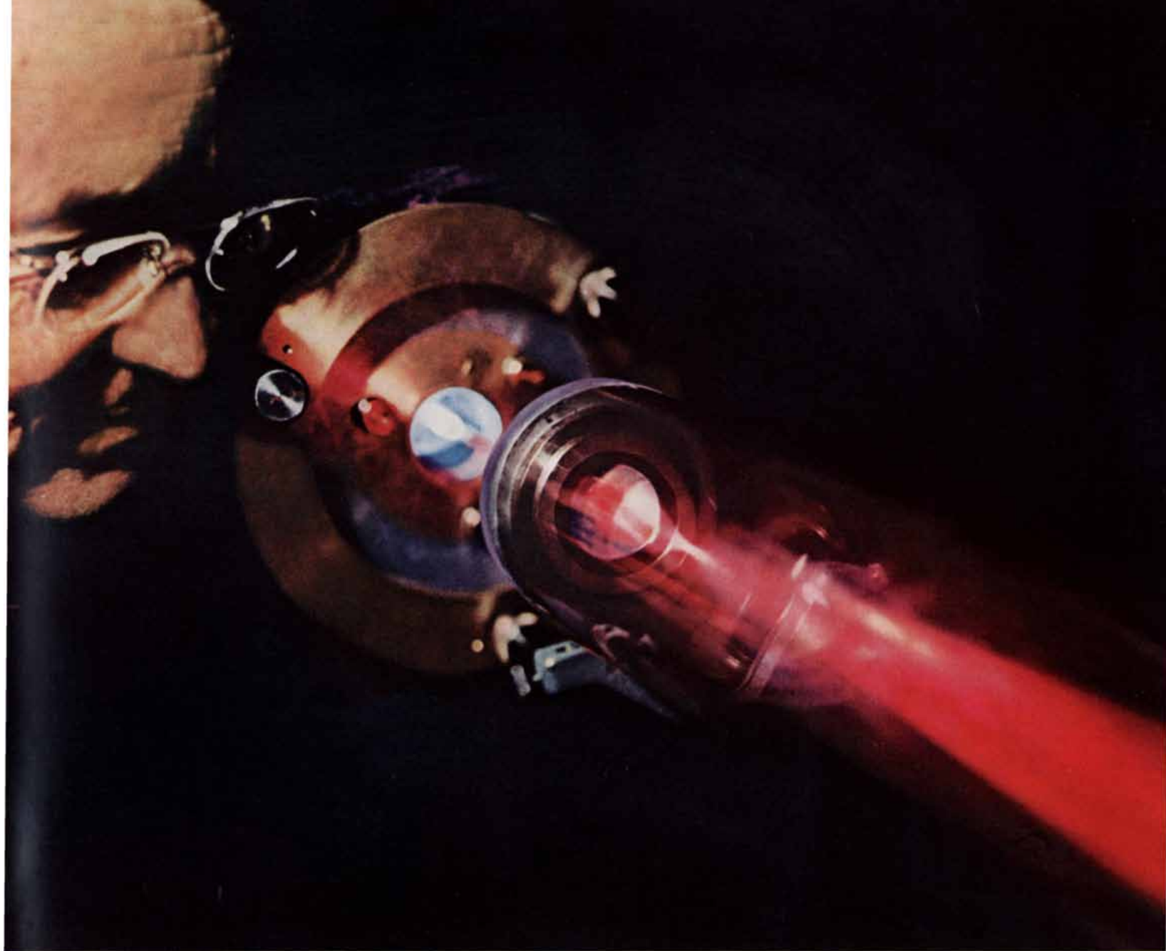
Helium-neon gas laser in action at the David Sarnoff Research Center, Princeton, N.J.
