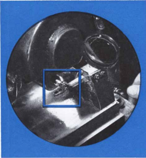
DIAMOND STYLUS engraves lines axially along barrel and cap of gold and silver pen and pencil sets at the A. T. Cross Co., Providence, Rhode Island. Specially built machines utilizing diamond tools were developed to increase the speed and precision of this operation.
