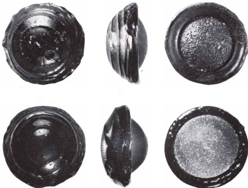
TEKTITE ABLATION and excellent imitation of it are shown in these photographs from the laboratory of Dean R. Chapman of the Ames Research Center at Moffett Field, Calif. Front, side and back views of an australite button tektite are seen in the top row. Similar views of an artificial tektite produced by Chapman in wind tunnel are shown in bottom row.
