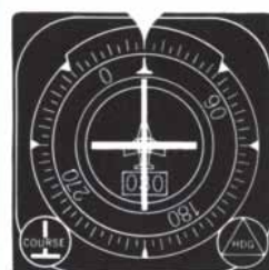
FLIGHT DIRECTOR INSTRUMENTS are the Horizon Director Indicator ( upper right in each panel ) and Course Deviation Indicator ( lower right in each panel ). In top panel they show aircraft to right of glide slope, as seen in plan view from above ( left ). It is also below the slope. Command bar ( color ) of horizon indicator tells pilot to turn right and go up. Course indicator shows him his position in relation to glide-slope and localizer beams. In middle, the aircraft is almost on course. At bottom it is fully on course.
