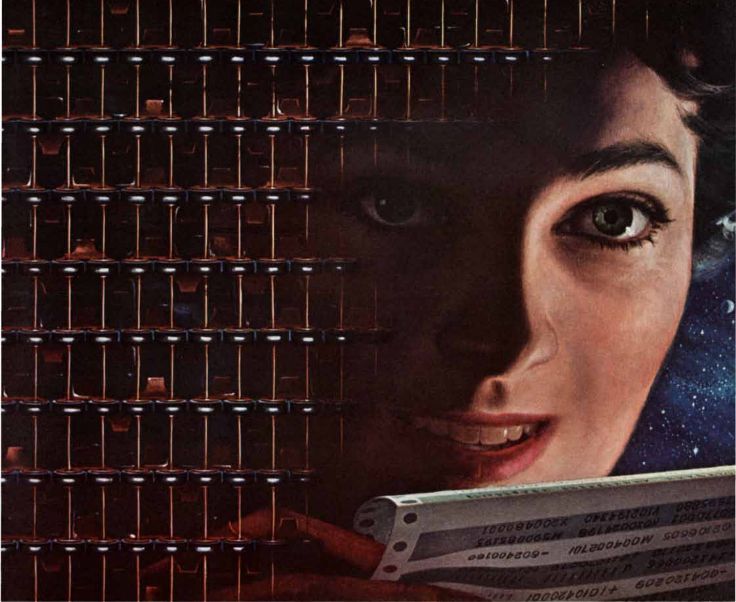
Enlarged view of a memory core plane used in electronic computers.
