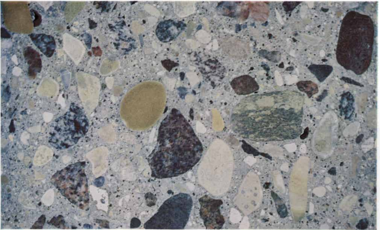
SECTION OF CONCRETE is shown approximately actual size. Pieces of coarse aggregate, consisting normally of crushed stone or gravel, and the grains of sand constituting the fine aggregate
