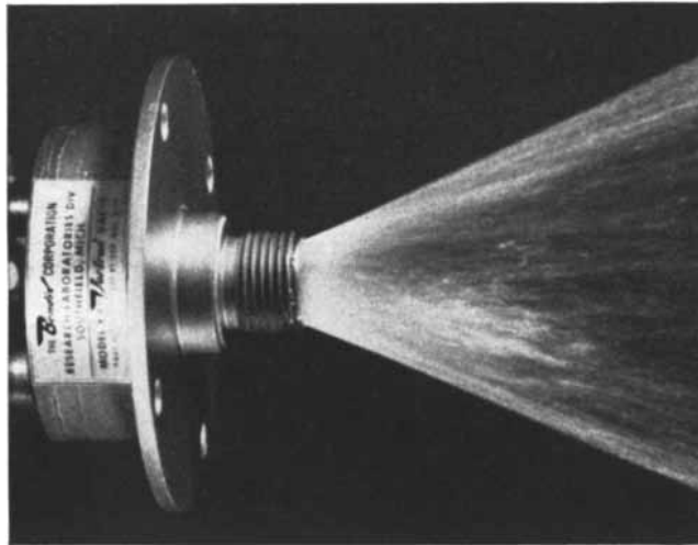
Vortex Valve for operation at 2000°F.
