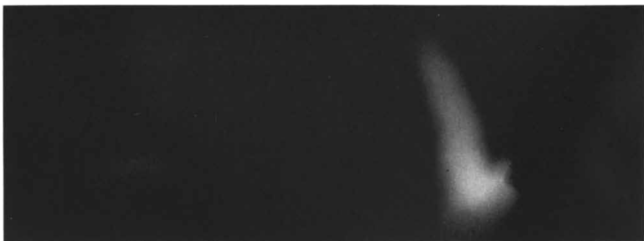
Spark crossing a gap in a 10-nanosecond exposure
