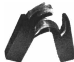
The key to the fracture behavior of ausform steels lies in the fibered structure which resists crack growth.
