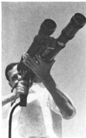
LASER RANGER IN GUN CONFIGURATION FIRES A LIGHT BEAM TO GIVE PRECISE RANGE OF OBJECTS UP TO TEN MILES AWAY — RANGE IS INSTANTLY READOUT BY OPERATOR.
