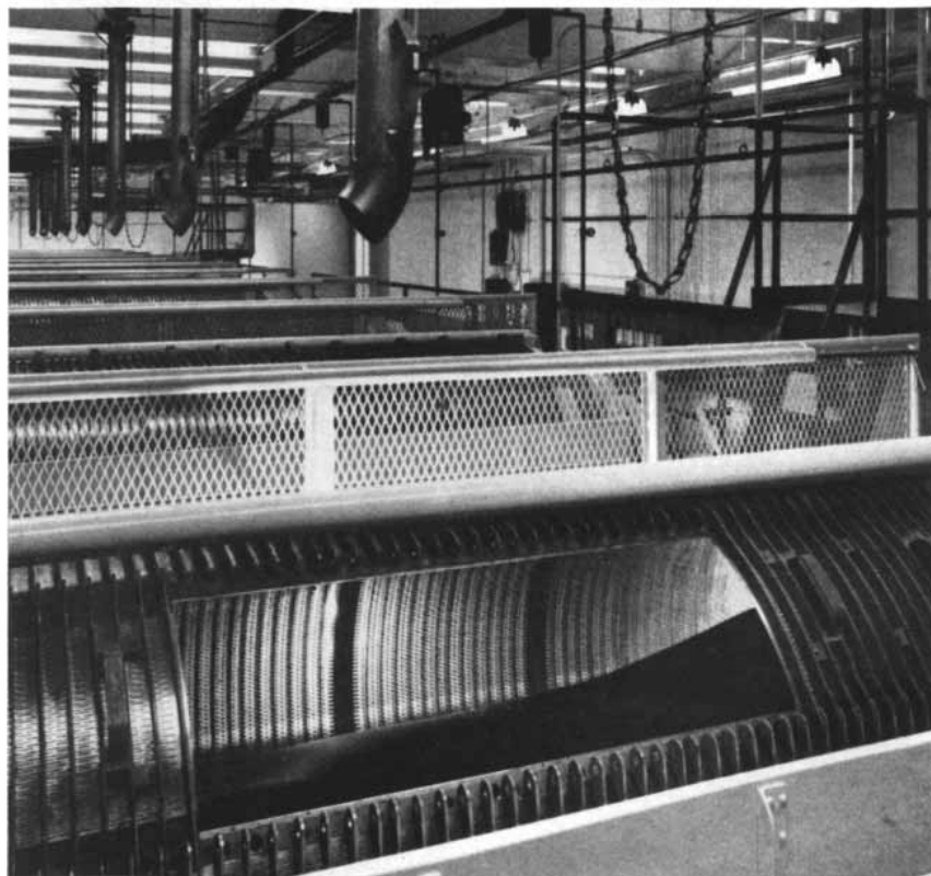
PRESSES receive crushed grapes from holding vats on the floor above through pipes ( top ). The black rubber bag visible inside the press in the foreground will be inflated with air, forcing residual skins and seeds to cling to the sides of the stainless steel cylinder.
