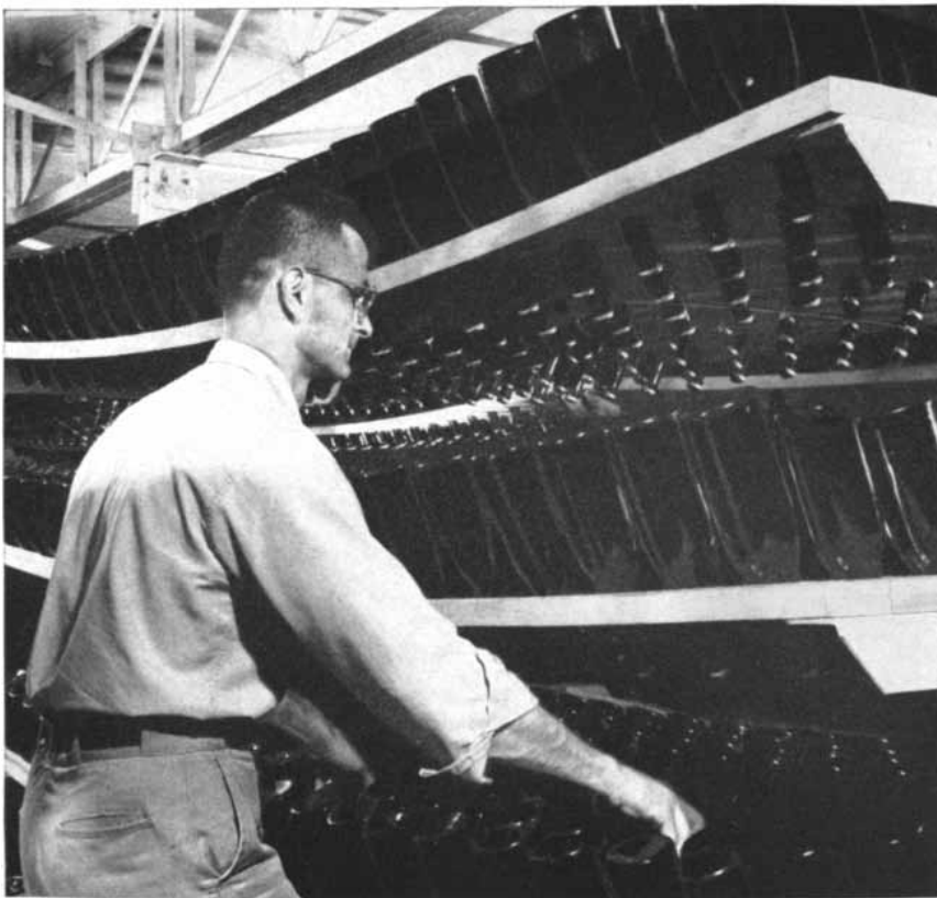
NEW BOTTLES containing domestic U.S. champagne are stacked on a "riddling" shelf of ash, counterpart of the French A-frame. Sediment accumulates in the neck and can be discarded by briefly uncorking the bottle. Both photographs were made at the Taylor Wineries.
