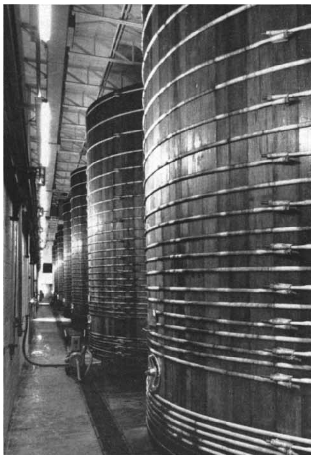
REDWOOD VATS house the aging wine and facilitate mellowing by admitting oxygen through redwood planks. These vats, photographed at the Taylor Winery, have a capacity of 63,000 gallons.
