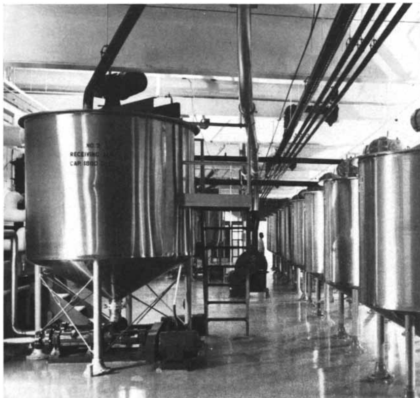
RECEIVING TANKS at left transfer must from a crusher on the floor above to the holding vats at right, enabling the winery to process the harvest of two types of grape. This photograph and the one below were made at the Taylor Winery in Hammondsport, N.Y.
