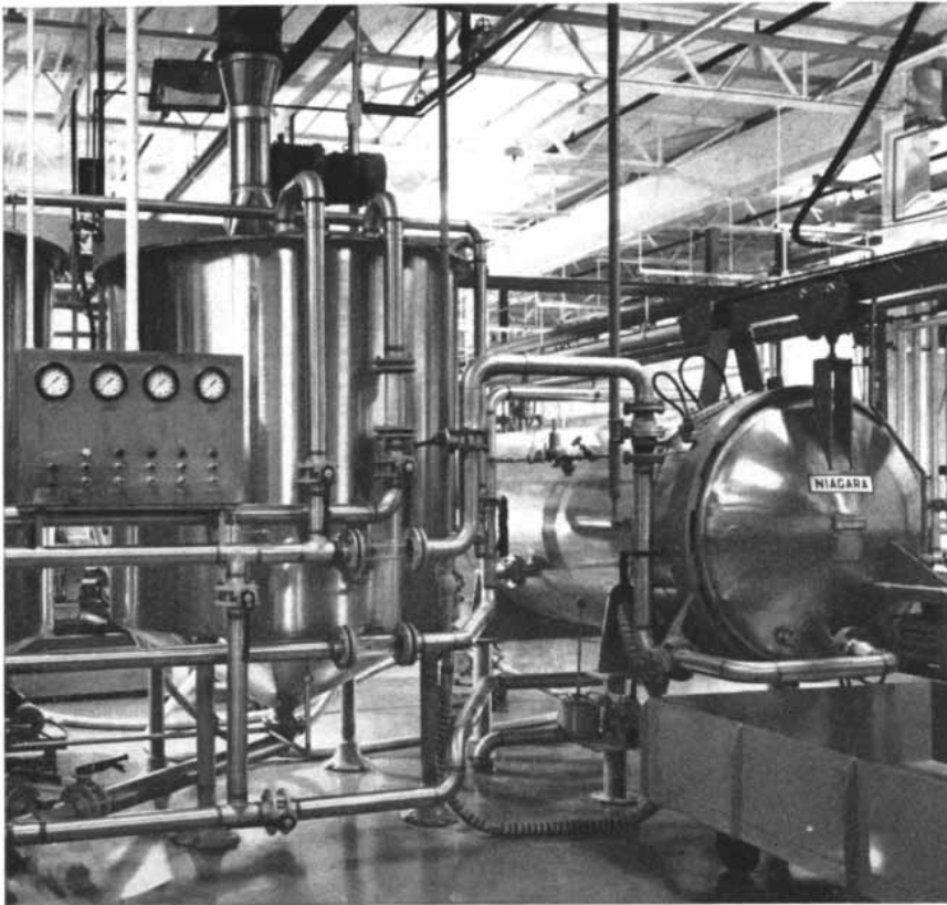
FILTERING UNIT shown at right in this photograph removes sediment from the wine in settling tanks ( left center ). Below the filter is a trough into which residue is dumped.
