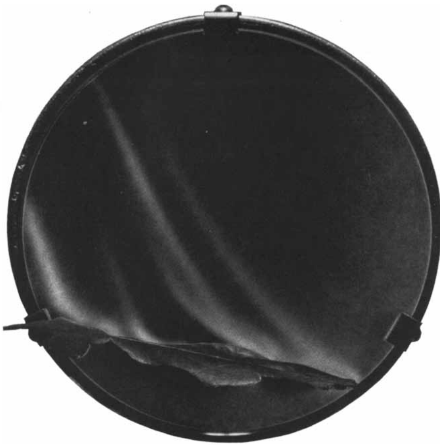
CONVECTION CURRENTS rise from a sun-warmed bur oak leaf. Sunlight could raise foliage to lethal temperatures except for the reradiation of solar energy and the cooling effects of transpiration and convection currents. The air movement, here revealed by schlieren photography techniques, causes an exchange of gases: water vapor and oxygen are carried away and fresh supplies of carbon dioxide are brought in. The photograph was made by David Gates of the National Bureau of Standards Boulder Laboratory.
