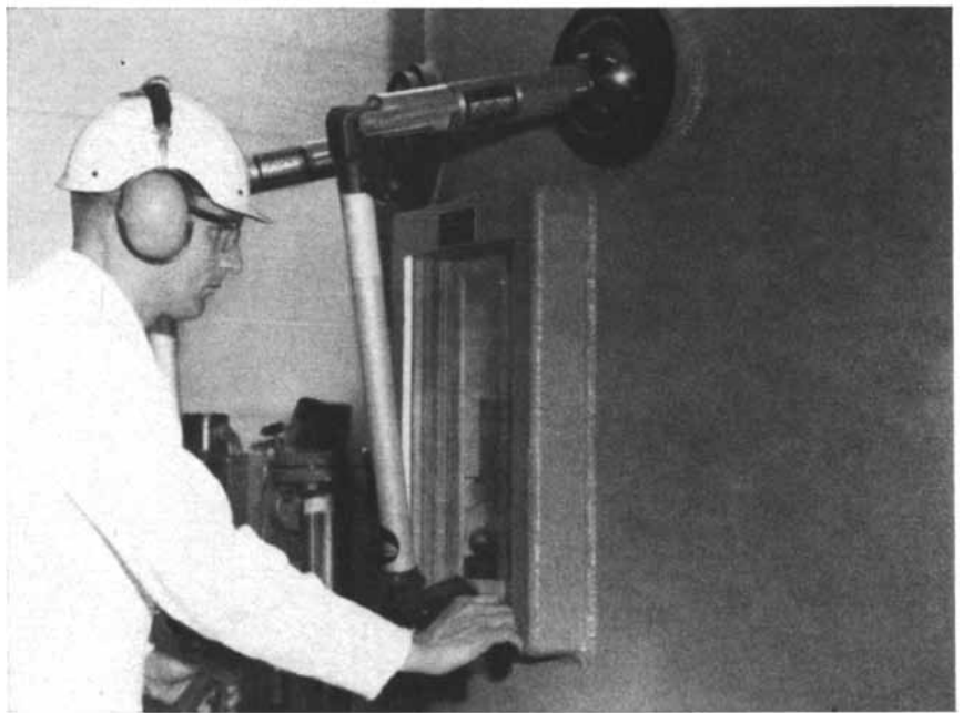
PROPELLANT STUDIES are conducted inside an armored cell with the aid of master-slave manipulators. This Mini-Manip installation is in Redstone Arsenal's Gorgas Laboratory.
