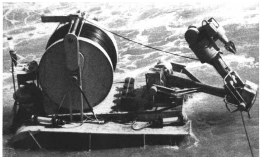
SUBMARINE MANIPULATOR, built for the U.S. Navy by General Mills, undergoes tests off the California coast. The Navy bathyscaphe Trieste is equipped with a similar grapple.
