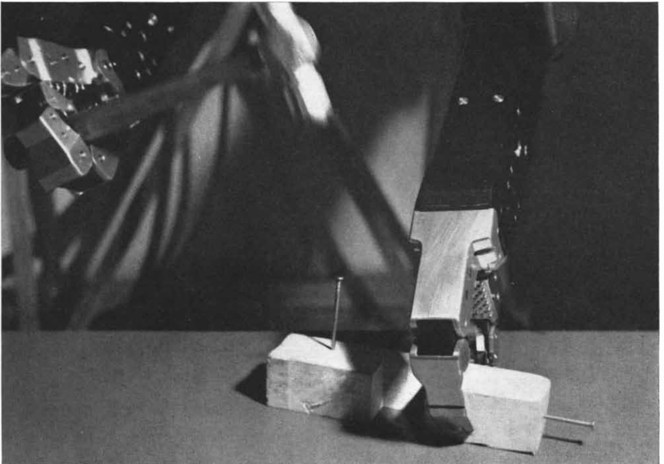
TEST OF DEXTERITY for the controller of Handyman involves holding and swinging a hammer with the manipulator's right
