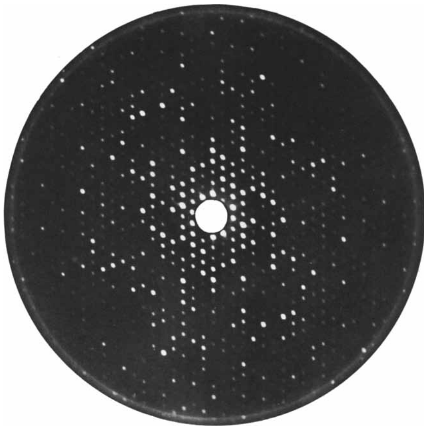
X-RAY DIFFRACTION PATTERN was made from a single crystal of hemoglobin that was rotated during the photographic exposure. Electrons grouped around the centers of the atoms in the crystal scatter the incident X rays, producing a symmetrical array of spots. Spots that are equidistant from the center and opposite each other have the same density.
