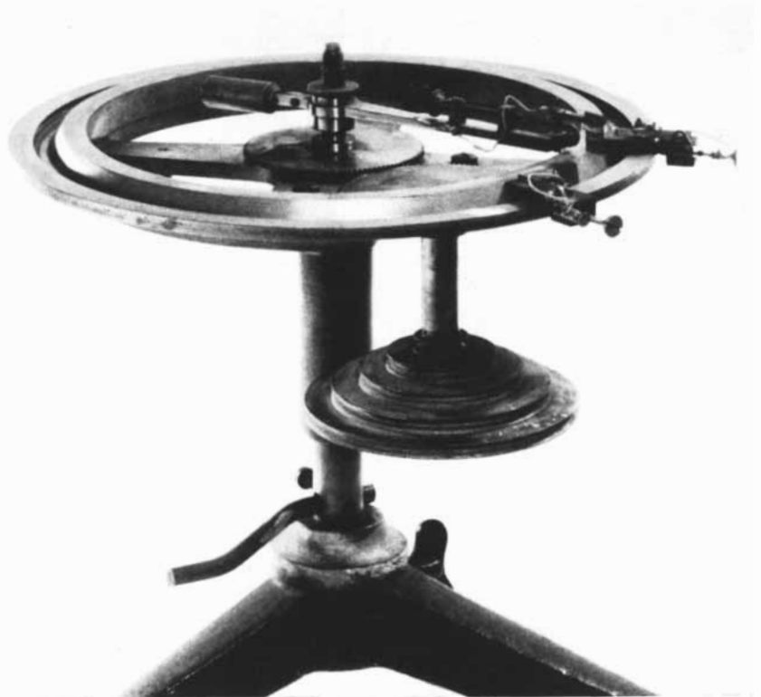
MEUMANN'S MACHINE is more fully shown. Time intervals set by the movable contacts shown in the illustration at the top of this page were recorded on a drum, as were subjects' responses. Among other things, Meumann sought to learn how such stimuli as sounds and lights delimiting an interval affected a subject's judgment of the duration of the interval.
