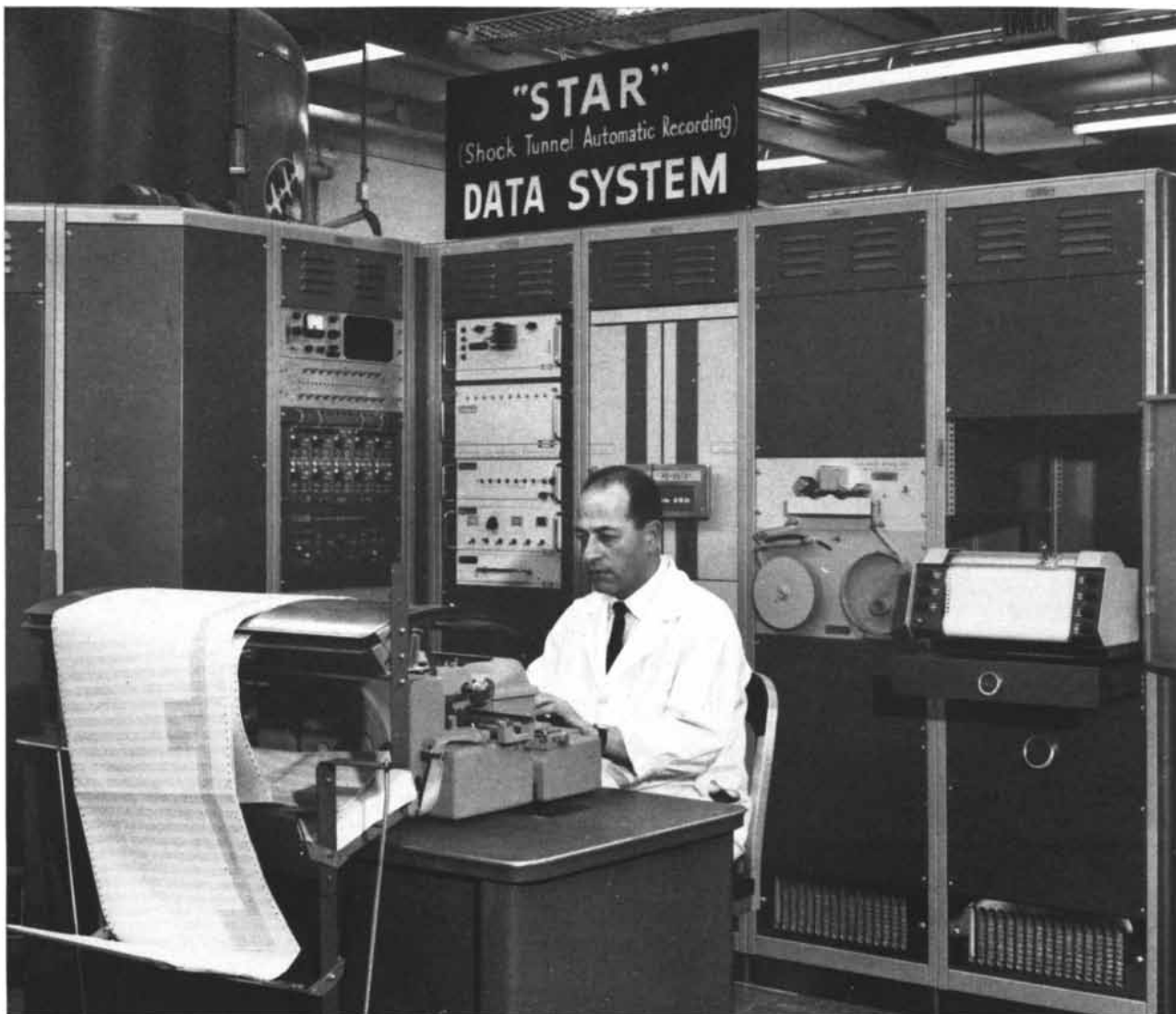
Republic Aviation's shock tunnel data system uses PB250 computer and Raytheon digital equipment
