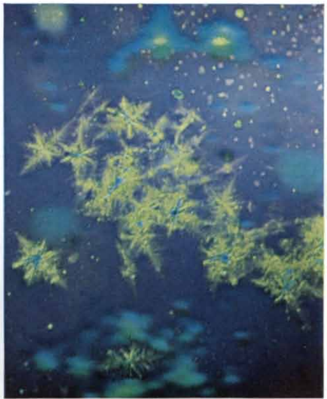
DENDRITIC CRYSTALS of polyethylene resemble similar crystals of snow. These crystals formed in a dilute solution of polyethylene that was rapidly cooled. Here they are flattened on the microscope slide; when they float, they curl up into spherical shapes.
