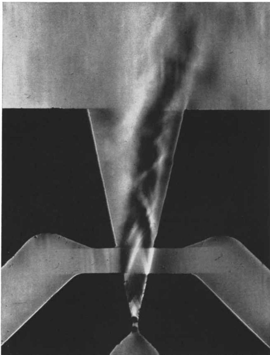
SCHLIEREN PHOTOGRAPH, made by an optical technique that detects density gradients in a gas flow, demonstrates Coanda effect. A high-energy stream of air is locked onto the chamber wall at right after being subjected to a short blast of air from control jet at left.
