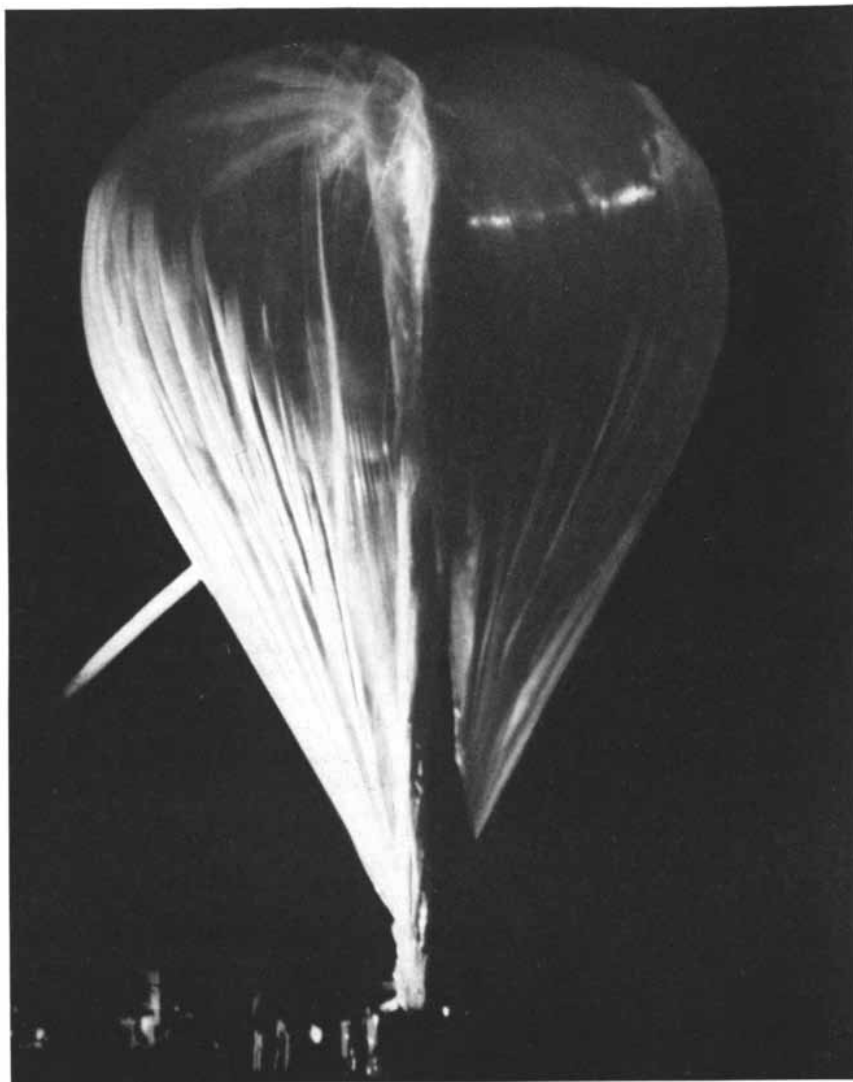
PREDAWN INFLATION of the polyester balloon proceeds under floodlights at Holloman Air Force Base, N.M., in preparation for the October 1964 observations of the cloud layer of Venus. Polyester proved a far more reliable balloon material than polyethylene.
