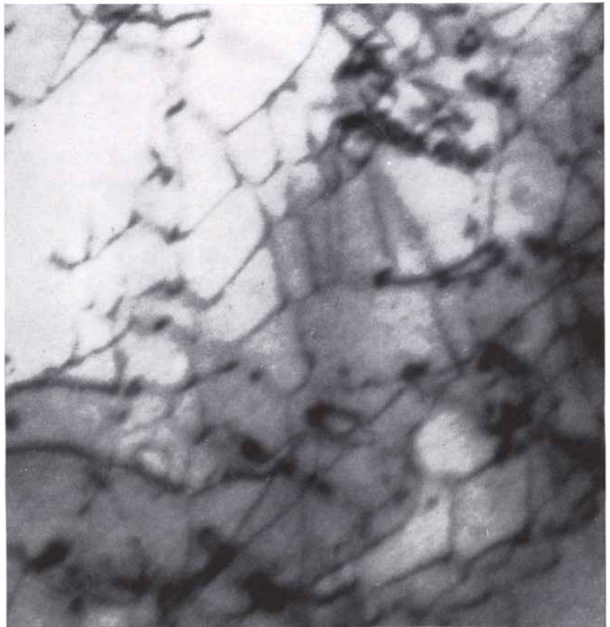
ENTANGLED DISLOCATIONS are shown in a crystal of iron, enlarged about 100,000 diameters. Entanglement is another structure that impedes motion of individual dislocations.
