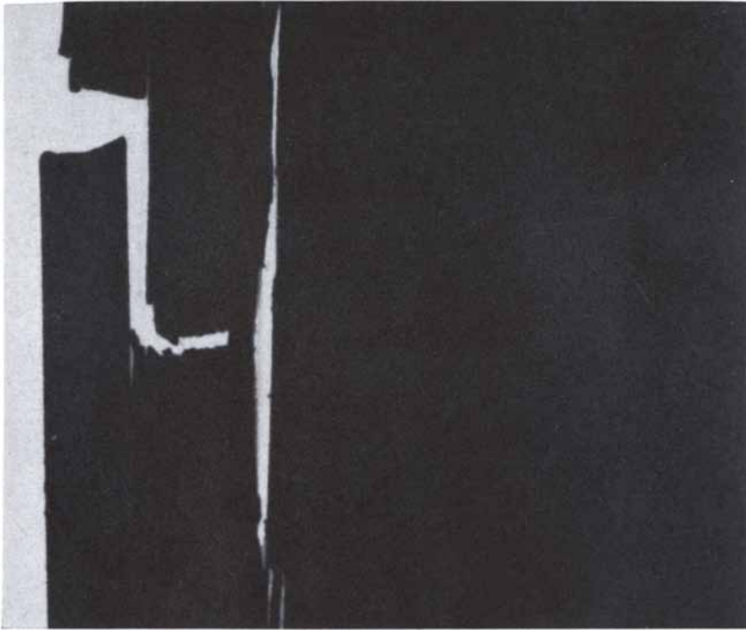
EFFECT OF CRACK in a material given high strength by fibers in a metal matrix is shown for silica fibers in copper. Forces at work are depicted in the illustration below.
