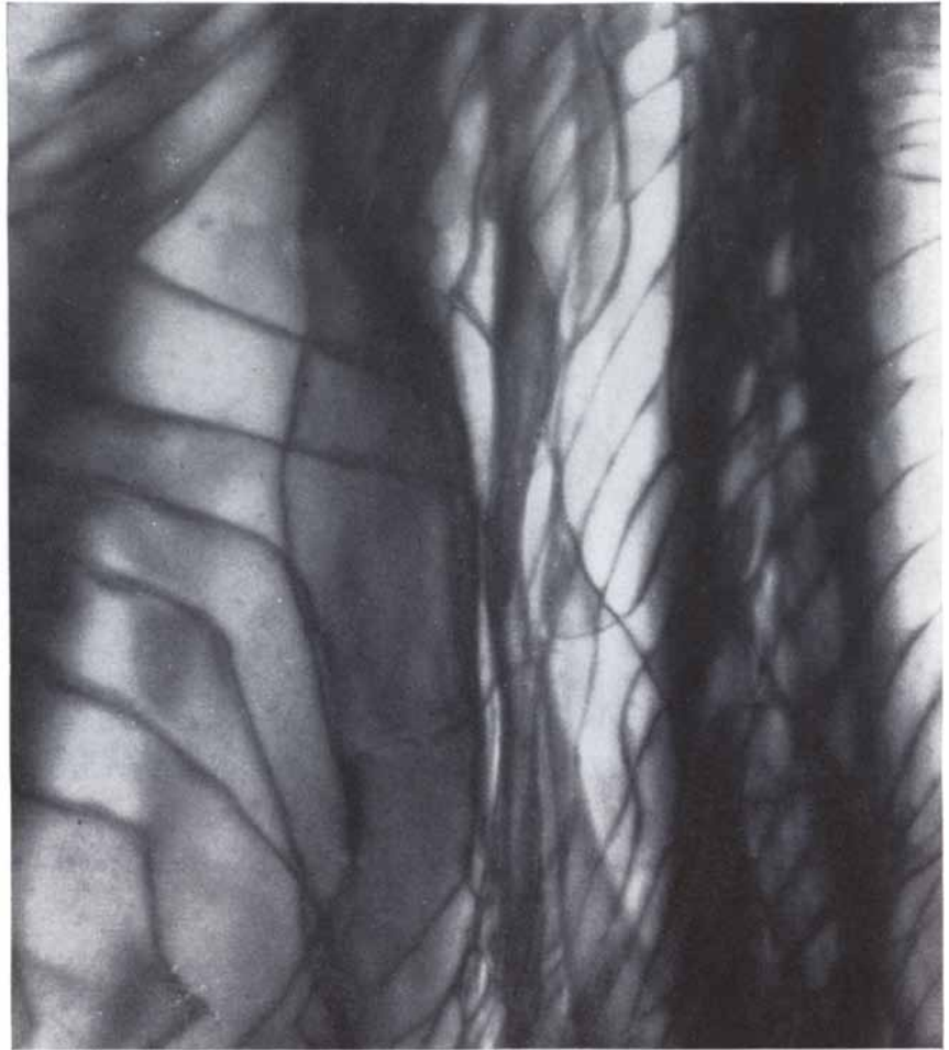
CERAMIC DISLOCATIONS, which move less readily than those in metal, appear in this view of a tungsten carbide crystal by electron microscope; enlargement is 88,000 diameters.
