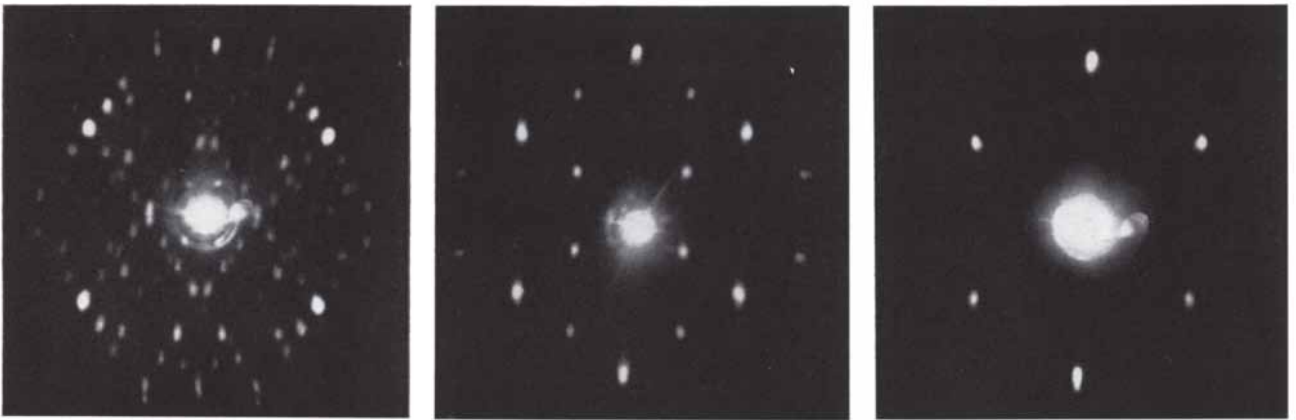
TUNGSTEN SURFACE at different stages of cleaning is shown in these three diffraction patterns. The patterns depict the (110) face of the crystal when it was bombarded with electrons having an energy of 75 electron volts. The pattern at left shows the badly contaminated surface before cleaning. The chief impurity is probably carbon. When the impurity was burned off by a short exposure to
