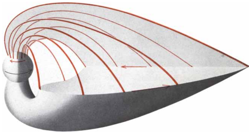
CONVECTION OF PLASMA within the magnetosphere is represented in this "closed tail" model. Plasma moves to the rear along the surface of the magnetosphere tail and returns up the center of the tail, pulling the polar-field lines with it. The ends of the field lines, which connect to the earth's auroral zones, set up ionospheric electric currents in polar regions. Motion of plasma is indicated by colored arrows in tail; colored arrow on earth shows corresponding movement of ends of polar-field lines. Black arrow shows rotation of earth.
