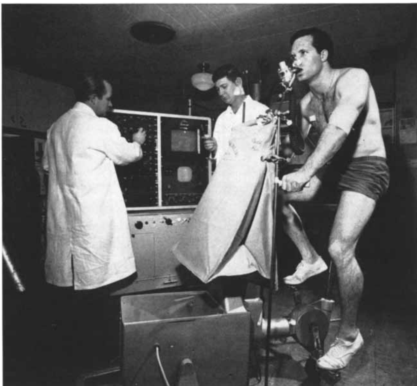
OXYGEN INTAKE is measured during controlled exercise on a bicycle ergometer. The air exhaled by the subject is collected in the bag to provide a basis for the calculation of how much air he inhaled. Electrocardiograms and other data are recorded on panel at rear.
