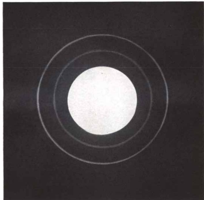
X-RAY PATTERNS OF IRON show how the crystal structure of iron varies with pressure. To provide a means for estimating pressure sodium chloride is mixed with the iron powder. At room
