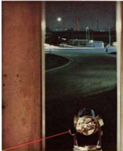
At top, approx. 1 per cent of transmitted beam is returned from retro-reflector. Note back-scatter from transmitted beam.
