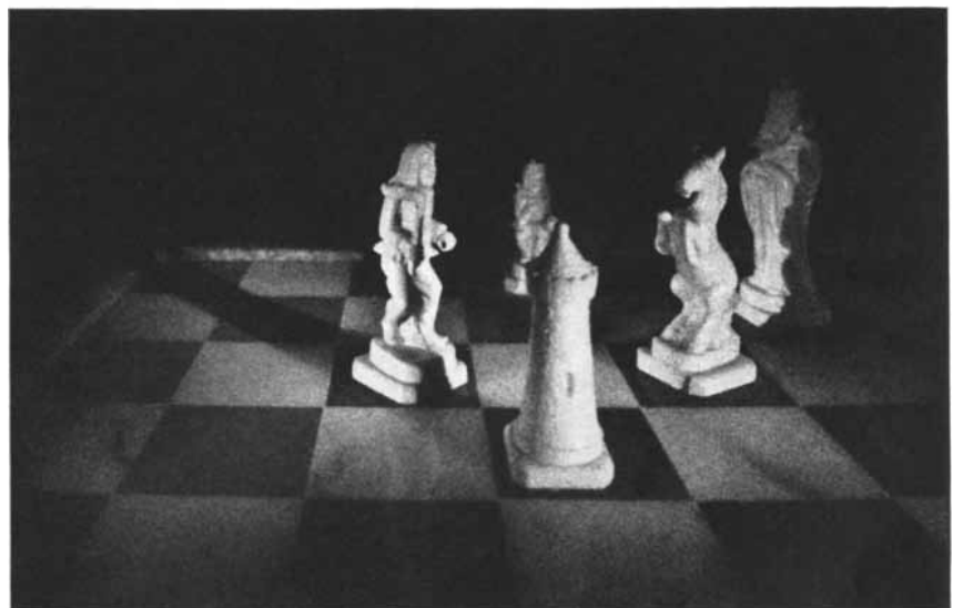
PARALLAX EFFECT is evident in these three virtual-image photographs, all made from the same hologram. The apparent displacement of the chessmen resulted from moving the hologram slightly. The same effect could have been obtained by keeping the hologram stationary and moving the camera or by keeping both stationary and moving the laser.
