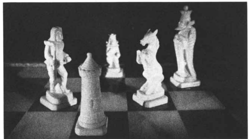
RECONSTRUCTED IMAGE was made by directing a laser beam through the hologram. The reconstructed waves were then passed through a lens and brought to a focus, thereby forming an image of original scene, even though chessmen had long since been removed.
