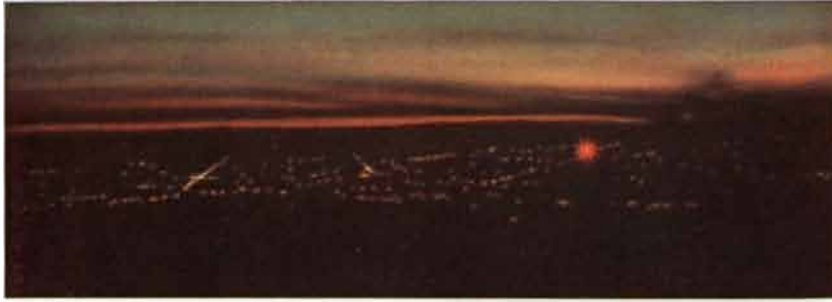
Distance: 25 miles; Power: 1/25th that of an ordinary flashlight; Alignment: slightly off beam axis to avoid overexposure.
