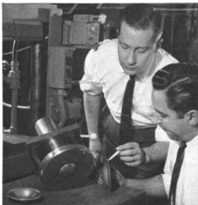
A. T. Spencer (left) and K. H. Pohl, originators of the structural laminate, demonstrate the results of postforming it with a heated die.
