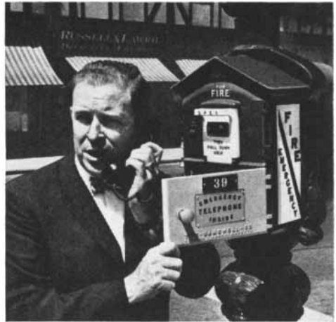
A Gamewell engineer tests new combination Code/Voice fire alarm and citizens' emergency reporting system developed by Bliss-Gamewell. System offers municipalities an effective, inexpensive way to better fire and police protection.
