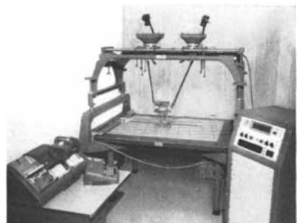
ECARS (Electronic Coordinatograph and Recording System) with input coordinatograph mounted on Stereoplottor. One of K&E's over 9,000 creative products for the creative engineer.
