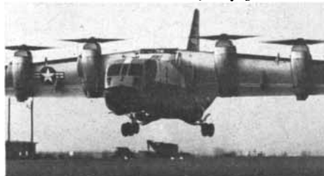
The XC-142A is the world's largest flying V/STOL.
