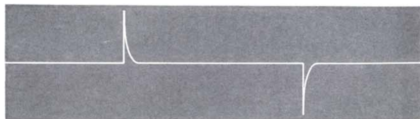
PIEZOELECTRIC EFFECT caused by stress on bone is illustrated. Each rectangle represents a piezoelectric crystal which, when compressed (2), produces an electric charge that tends to "leak" (3). When stress is removed (4), crystal resumes its original shape and charge is reversed. These steps give rise to oscilloscope trace of shape shown at bottom.
