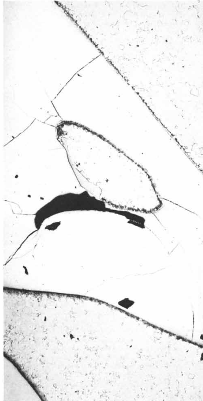
black outline is iron carbide. In a heavily shocked, diamond-bearing Canyon Diablo meteorite ( middle ) the alpha iron is in the form of many small crystals. A fuzzy darkened area around the iron carbide shows that carbon diffused into the metal while it was in the gamma state and rapid cooling con-
