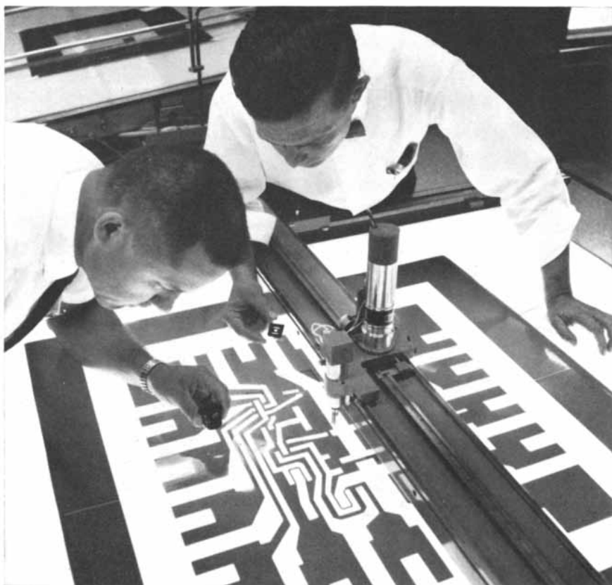
PRECISION MASK for laying down the pattern of elements in an integrated circuit is drawn on a large scale by a computer at Western Electric. By means of precision photographic lenses the mask is reduced to microscopic size and replicated as may be required to cover the surface of a silicon wafer. The overall reduction in scale is about 500 to one.
