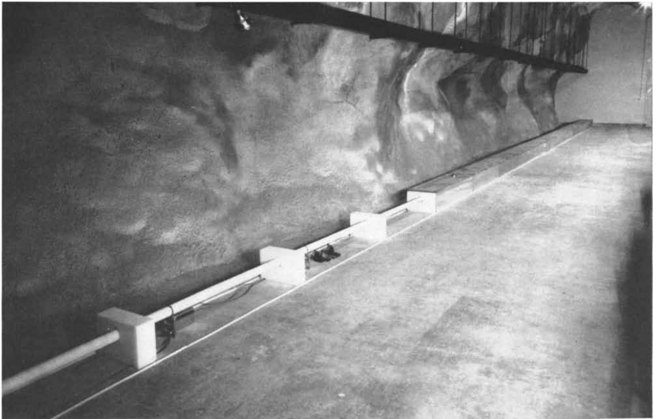
QUARTZ ROD of a strain seismograph installed at the Cal Tech facility on Oahu, Hawaii, is shown in this photograph. The rod is
