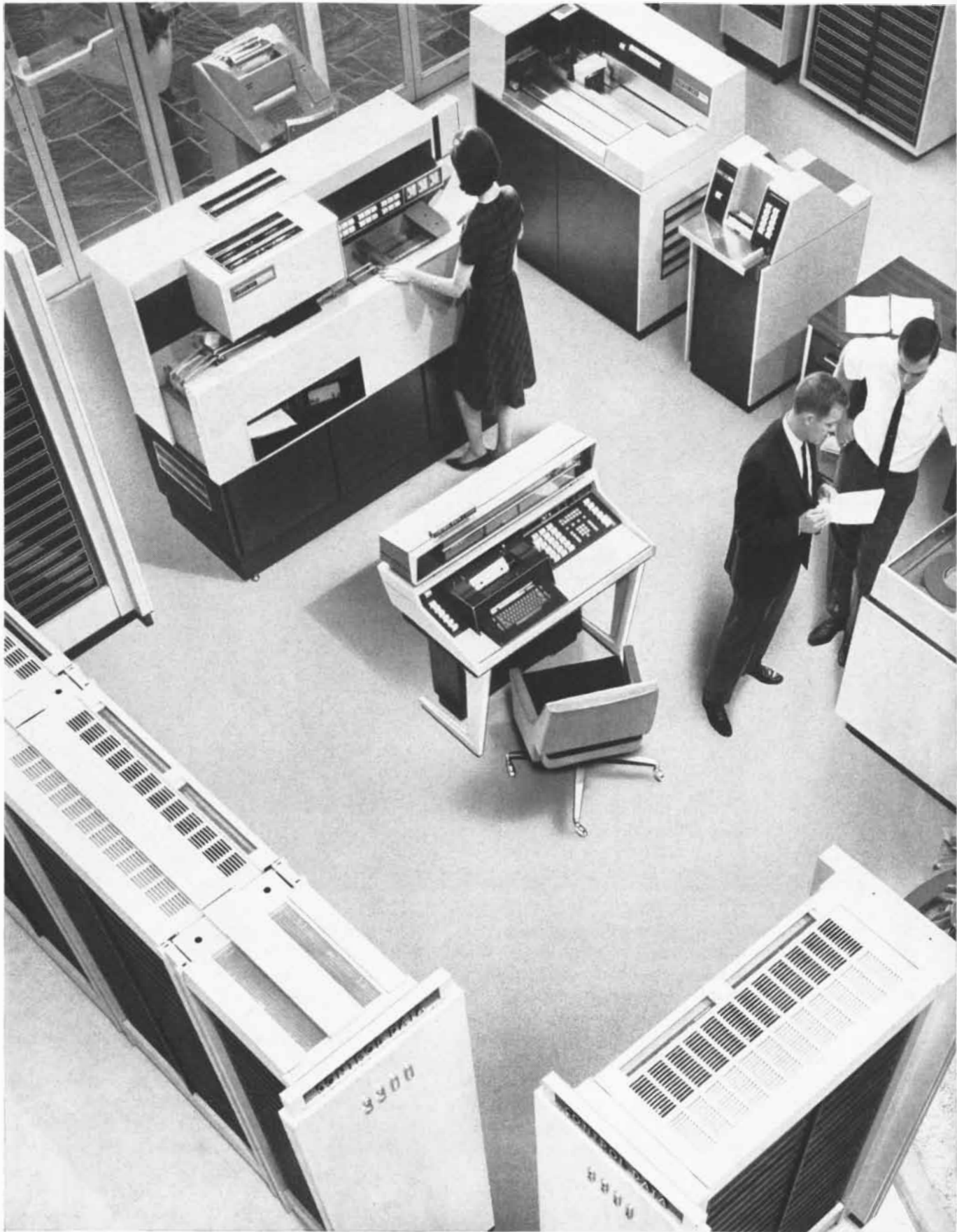
CONTROL DATA 3300 Time Sharing System shown here includes the following peripheral devices: 915 Page Reader, 405 Card Reader, 415 Card Punch, 852 Disk Storage Drive, 210 Entry and Display Station, and Tape Transports
