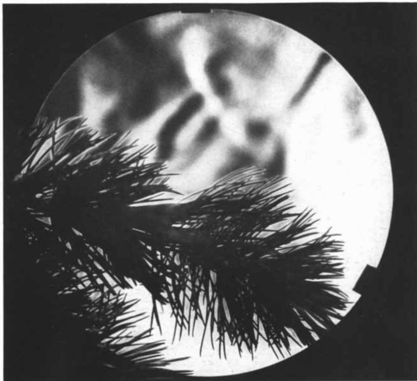
WARM PINE BRANCH is cooled by rising convection currents. Each needle yields some of its heat conductively to the cooler air in contact with the needle surface. As the air is heated it rises ( shadows above the branch in this schlieren photograph ). Cool air replaces it and repeats the process. The rising current is somewhat turbulent because of a slight wind.
