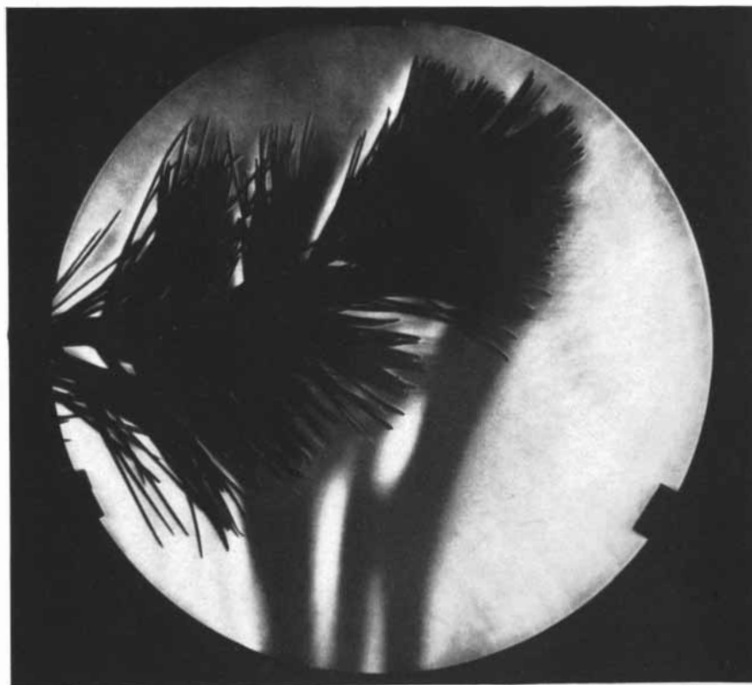
COOL PINE BRANCH that has lost heat by radiation to the night sky is warmed by falling convection currents. Each needle now absorbs heat from the warmer air in contact with its surface. As the air is cooled it sinks ( shadows below the branch in this schlieren photograph ). In both examples the heat transfer helps to stabilize the plant's temperature.
