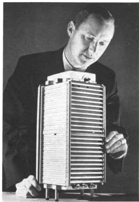
Radiation Cooled Fuel-Cell Module. Note that one set of louvers is open and one set is closed to illustrate how the effective emissivity is varied.
