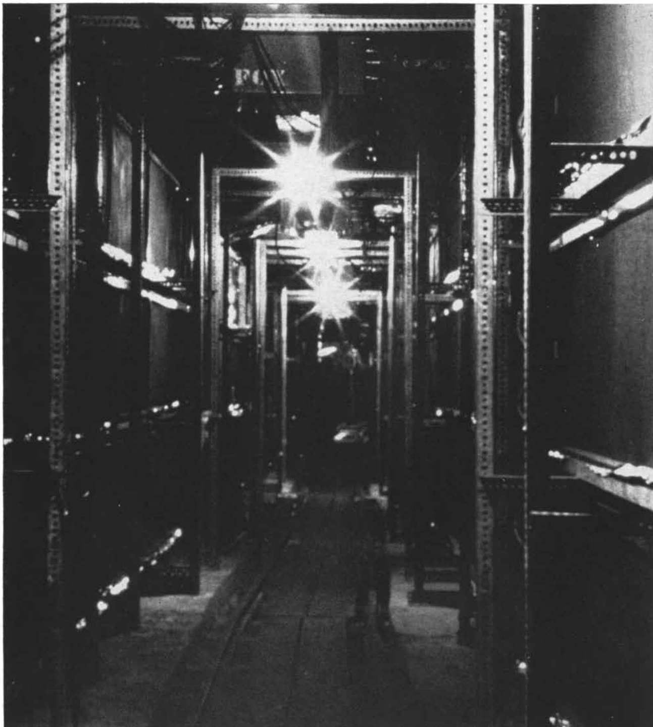
UNDERGROUND LABORATORY for detecting high-energy neutrinos from the atmosphere was hewn out of solid rock at a depth of 10,492 feet in a gold mine operated by the East Rand Proprietary Mines near Johannesburg. The laboratory is operated by physicists
