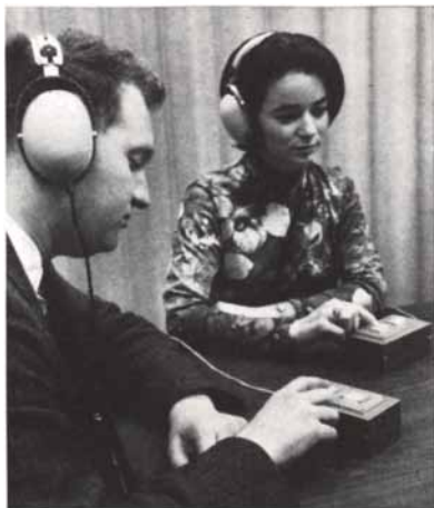
Test subjects listening to telephone channels of varying quality. Subjects heard test sentences transmitted over pairs of channels; for each pair they indicated, by pressing a button, which of the two they preferred. Signals from buttons were used to key-punch cards, which were then processed with adaptations of the "subjective space" program developed at Bell Laboratories.
