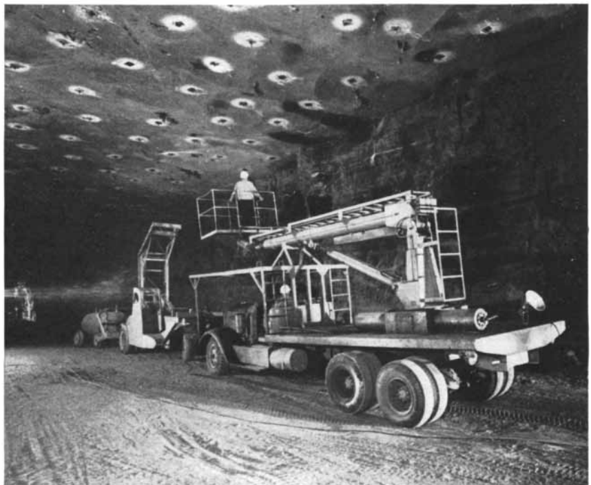
SHALE DEPOSITS will probably be mined in Colorado by techniques developed by the Bureau of Mines. Large underground "rooms" are mined by drilling, blasting and loading with heavy equipment. The bolts and plates in the roof lessen the likelihood of cave-ins.
