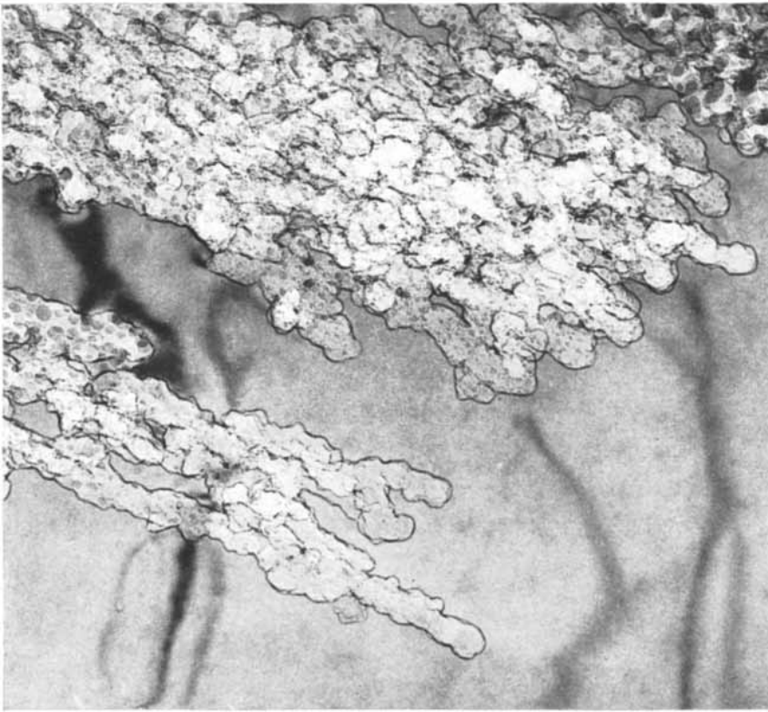
CORROSION TUNNELS develop from pits on the surface of an alloy that elongate in the direction of closest atomic packing ( toward bottom right in this case ). Tunnels are some 250 atoms in diameter; this micrograph of an alloy enlarges them some 100,000 diameters.
