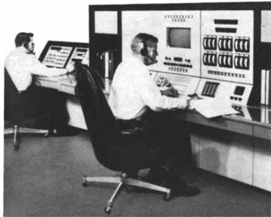
In NASA's tracking network. During manned space flight, Bendix-built consoles give a detailed, running report of each astronaut's physical condition and the operational performance of the spacecraft.
