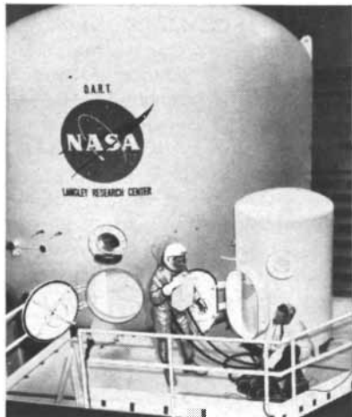
This sealable structure contains the prototype of a life-support system which includes facilities to maintain four men in space for a year.
