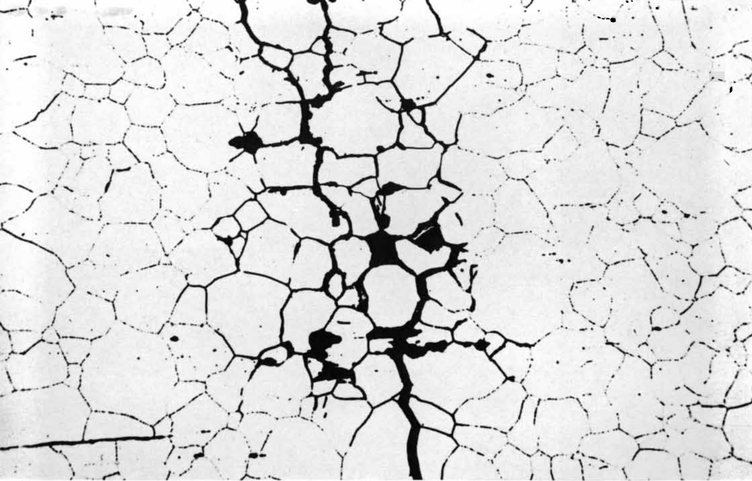
INTERGRANULAR CRACK caused by stress-corrosion appears as a network of heavy black lines running between the grains of a specimen of stainless steel in the photomicrograph above. The crack arises at the top. The specimen is enlarged 400 diameters.
