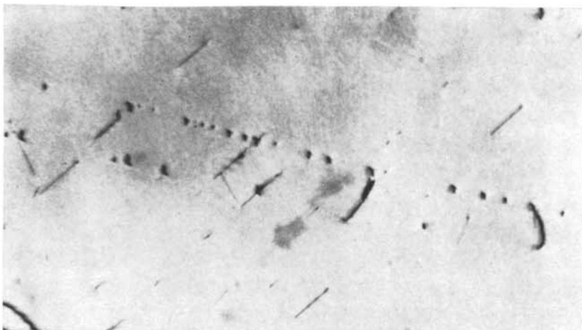
EARLY EFFECT OF CORROSION , the formation of pits ( rows of black dots ), is shown directly on the surface of a stainless steel. The dislocations ( black lines ) create slip steps that serve as nuclei for pits. The slip steps themselves cannot be seen in this micrograph.
