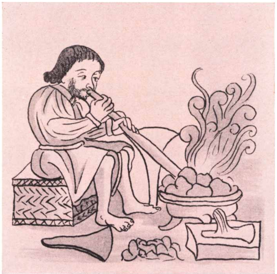
AXE-BLADE CASTING as practiced in Mexico is depicted in Bernardino de Sahagún's study of pre-Columbian technology. Copper was brought to melting temperature with a blowpipe; the molten metal ran out of a furnace tap into a stone mold. On the ground is a finished axe blank; this will be given its final form by hammering (see illustration below).
