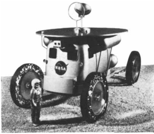
Exploring space. This scale model of a mobile lunar laboratory designed by Bendix for NASA would be capable of supporting two astronauts for two weeks of lunar exploration.
