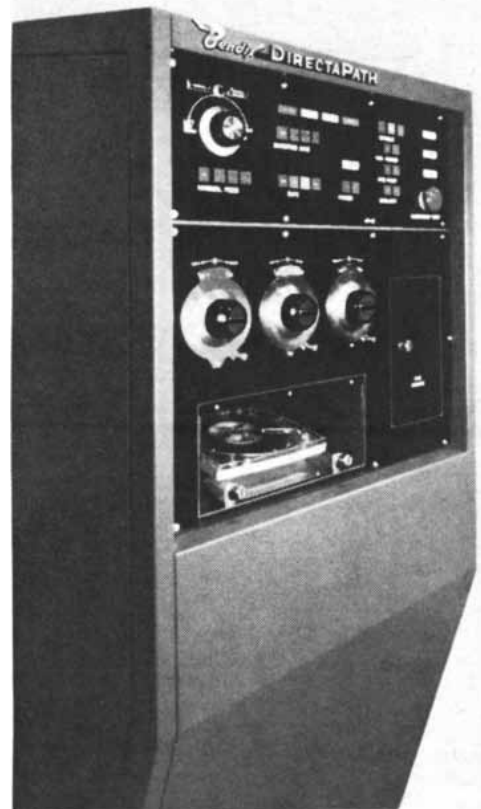
Increasing your buying power. Equipment such as the Bendix DirectaPath® that "plays" a magnetic tape to control metalworking machines, helps manufacturers increase production and improve quality to give you greater product value.
