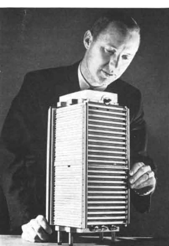
Radiation Cooled Fuel-Cell Module. Note that one set of louvers is open and one set is closed to illustrate how the effective emissivity is varied.
