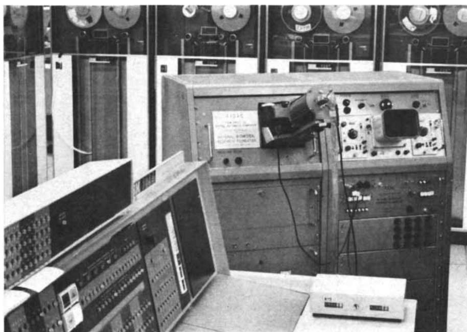
COMPUTER AND SCANNING DEVICE used by the authors are located at the Goddard Space Flight Center outside Washington, D.C. The IBM 7094 computer ( foreground ) receives descriptions of photomicrographs of chromosomes from the FIDAC scanner ( background ), on the basis of which it counts, analyzes and collates data on the chromosomes.
