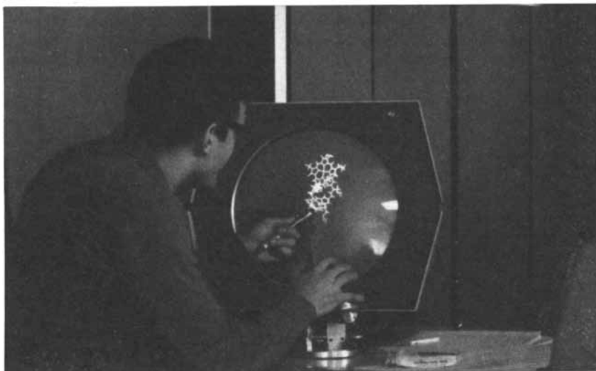
DISPLAY UNIT designed by John Ward and Robert Stotz has access to the large time-shared central computer at the Massachusetts Institute of Technology. The investigator communicates with the computer by typing commands or punching preset buttons on a keyboard or by pointing with the light pen. He regulates the direction and the speed of rotation of the model by moving the gimbaled control on which his right hand rests.
