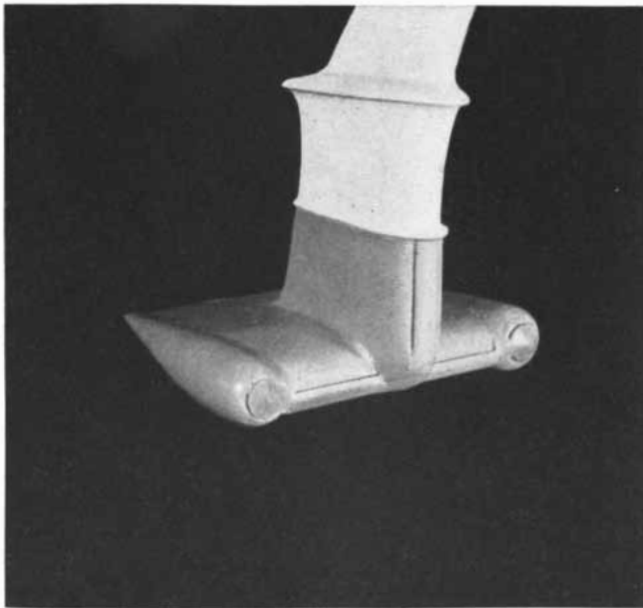
KEY PART of the hydrofoil is this foil with several slits for achieving the Coanda effect. Water emerging from the slits ( right )
