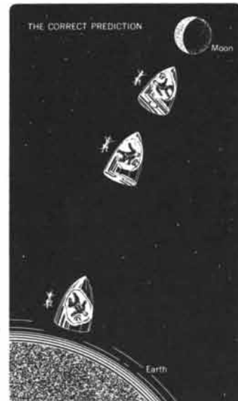
Fig. 3,B. Correct prediction is that a passenger would float with respect to the projectile during the entire trip. Verne was correct about the motion of the dog.
