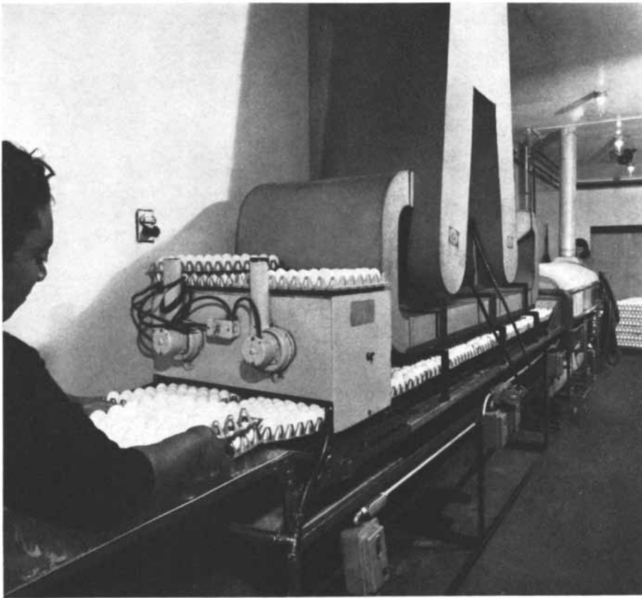
WASHING EGGS is one of the final steps en route to market. After leaving the washing machine eggs often receive light coating of oil to reduce evaporation before consumption.
