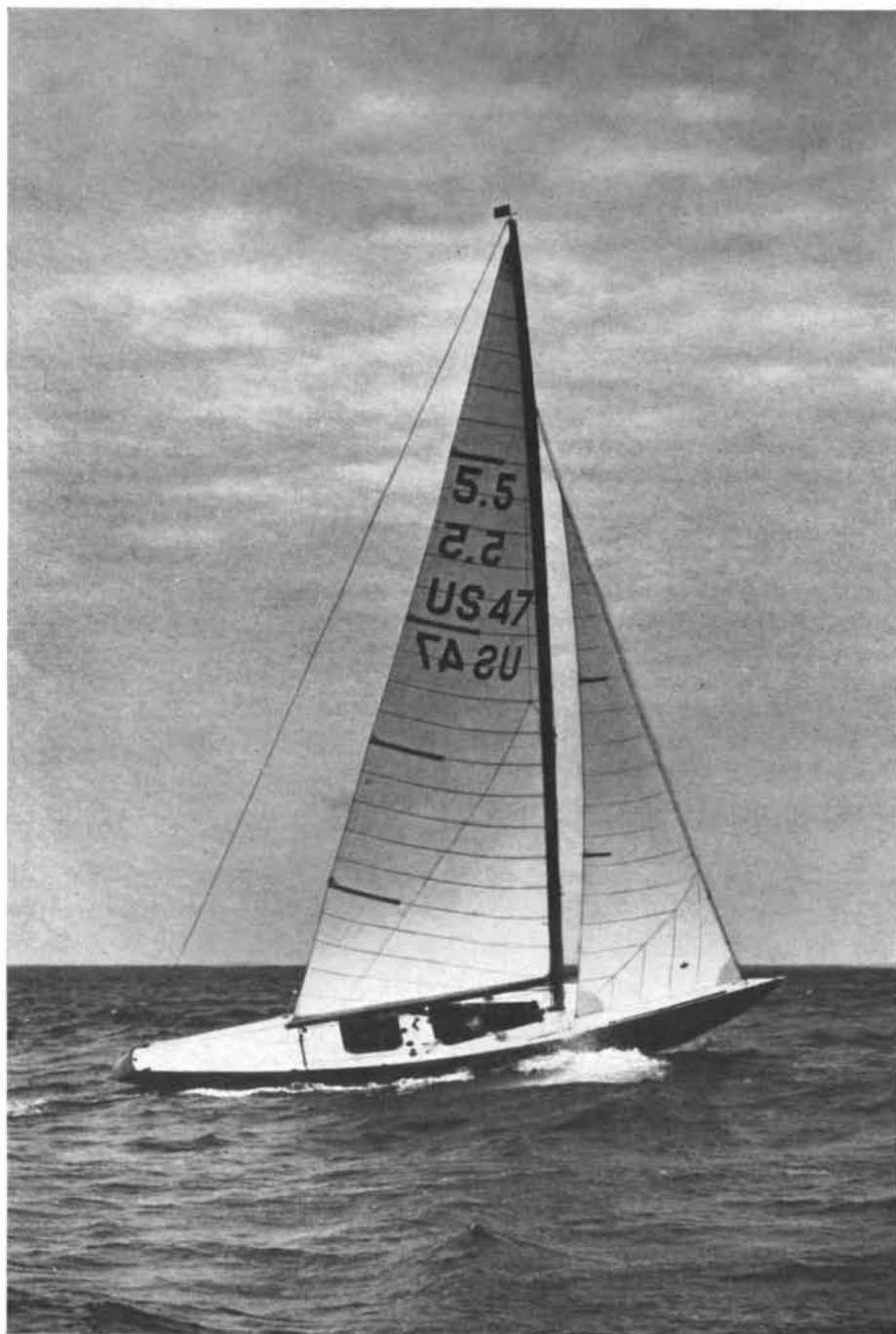
ANTIOPE RACING sails to windward in an international race. The wind is about 40 degrees off the bow; the sails are trimmed almost flat with a small angle of attack to the wind.
