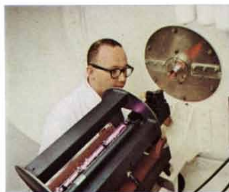
At the bottom of a steel-jacketed, 30-foot well, SLAC's Model 115 gas laser, which operates continuously for periods as long as 2000 hours, is checked by alignment technician Jack Higgins.
