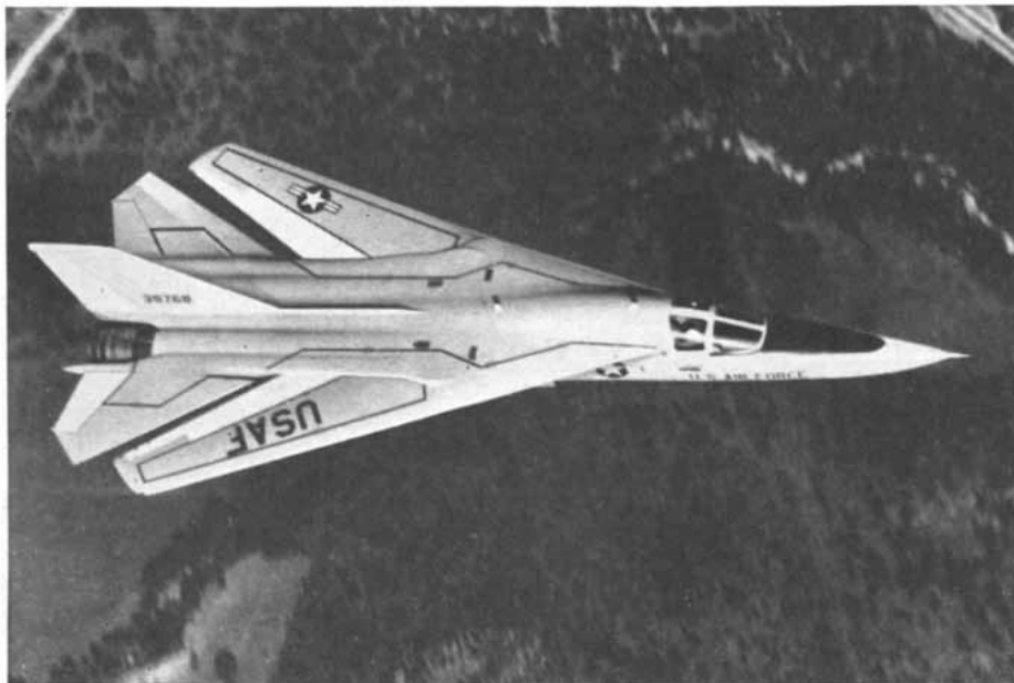
Top: The F-111 with its wings extended straight out for high lift at takeoff. Bottom: Wings being swept back to allow F-111 to reach supersonic speeds.
