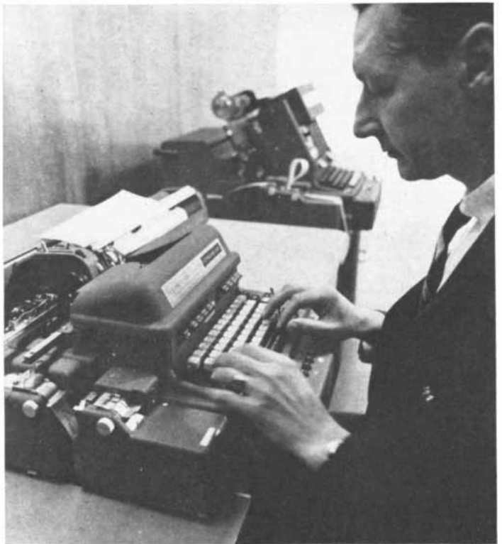
Semi-automatic system for making schematic drawings, eliminates hours of laborious hand work.
