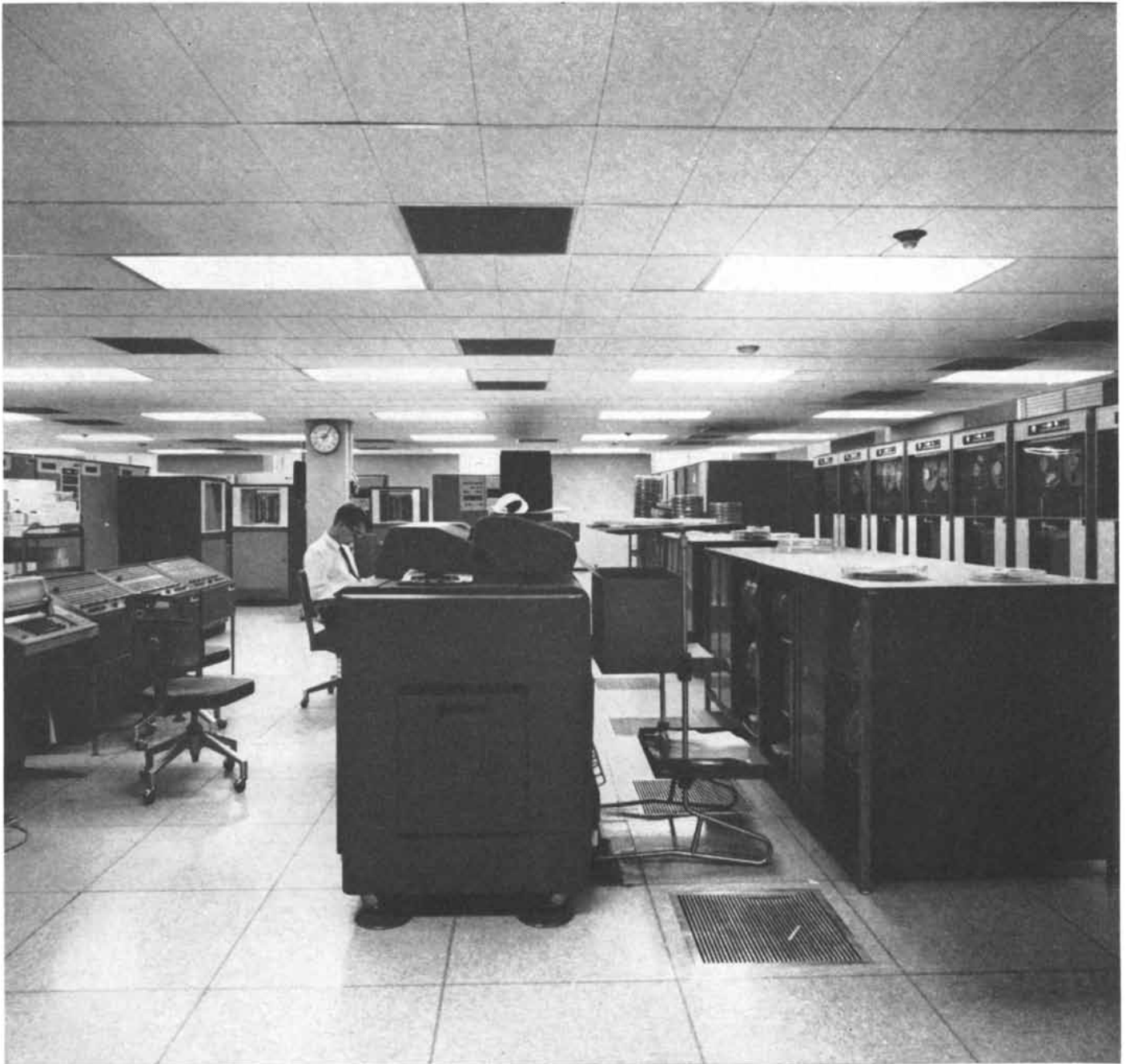
COMPUTER ROOM at M.I.T. houses the IBM 7094 central processing unit, memories and other central units of the Project MAC
