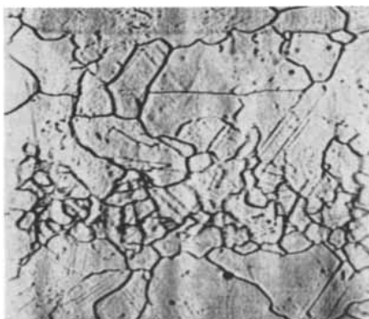
SURFACE ETCH PATTERNS for two argon crystals grown identically in all respects but growth rate are compared. The more quickly grown crystal ( right ) shows smaller average grain sizes and more slip lines than the more slowly grown crystal ( left ). It is from such photographs that one determines optimum growth conditions for large single crystals.
