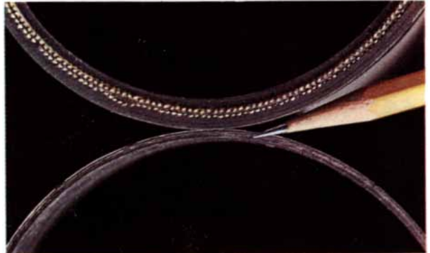
Wall thickness of new military hose with fiber glass reinforcement is less than one-third that of conventional military hose, yet burst strength is up to 50 percent higher.
