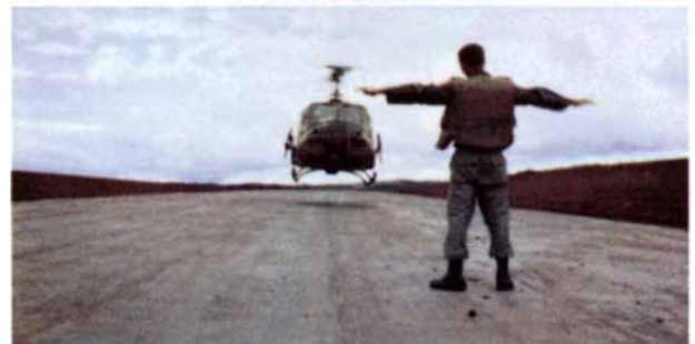
Major purpose of rubber landing mat is to eliminate dust kicked up by whirling helicopter blades.
