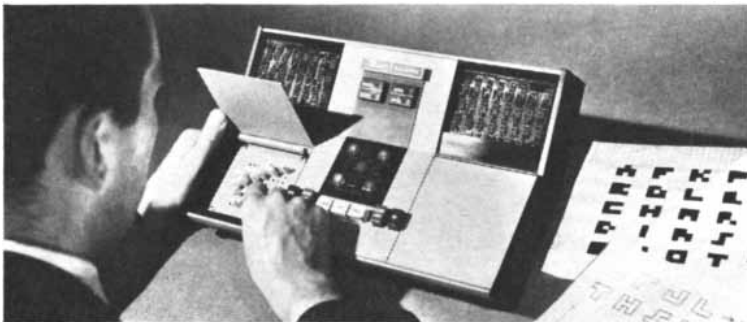
Helping machines learn. Using a punish and reward process, the operator is training a Bendix Pattern Recognition Device to classify letters of the alphabet. Such trainable systems are expected to have applications in manufacturing, aerospace controls and automation.
