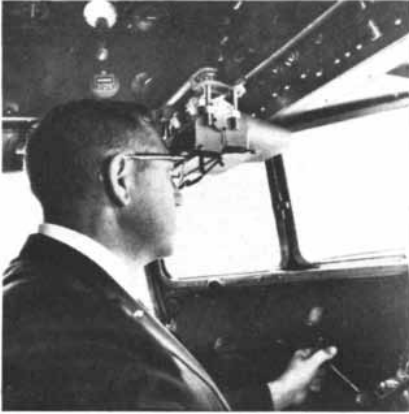
Giving a pilot another set of eyes. With a Bendix "Head-Up" display device, a pilot can see all the flight and landing information he needs in visual form, at the precise time he needs it—without lowering his head.
