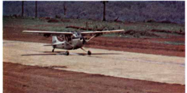
Observation plane lands on rubber-coated nylon mat. Uniroyal makes surfaces like this for military and civilian use.
