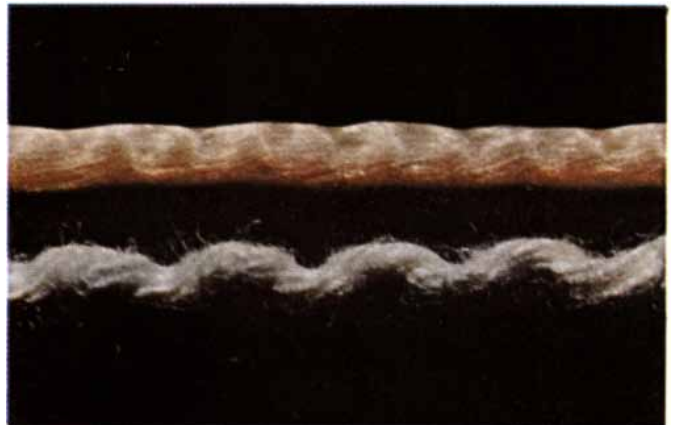
Strength member from single-ply belt (top) retains much more of its inherent strength because it is not crimped and bent during weaving like conventional ply (bottom).
