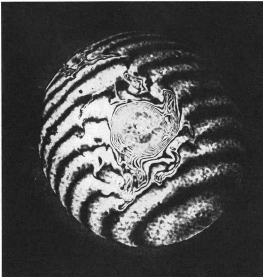
UNSTABLE PLASMA is made visible in this photograph produced by passing a laser beam through the plasma. The dark and light fringes resulting from interference of the light waves are displaced by inhomogeneities in the plasma. The photograph shows a common type of interchange instability called a "flute" instability. The phenomenon occurred in a "theta pinch" experiment conducted by Fred L. Ribe at the Los Alamos Scientific Laboratory.
