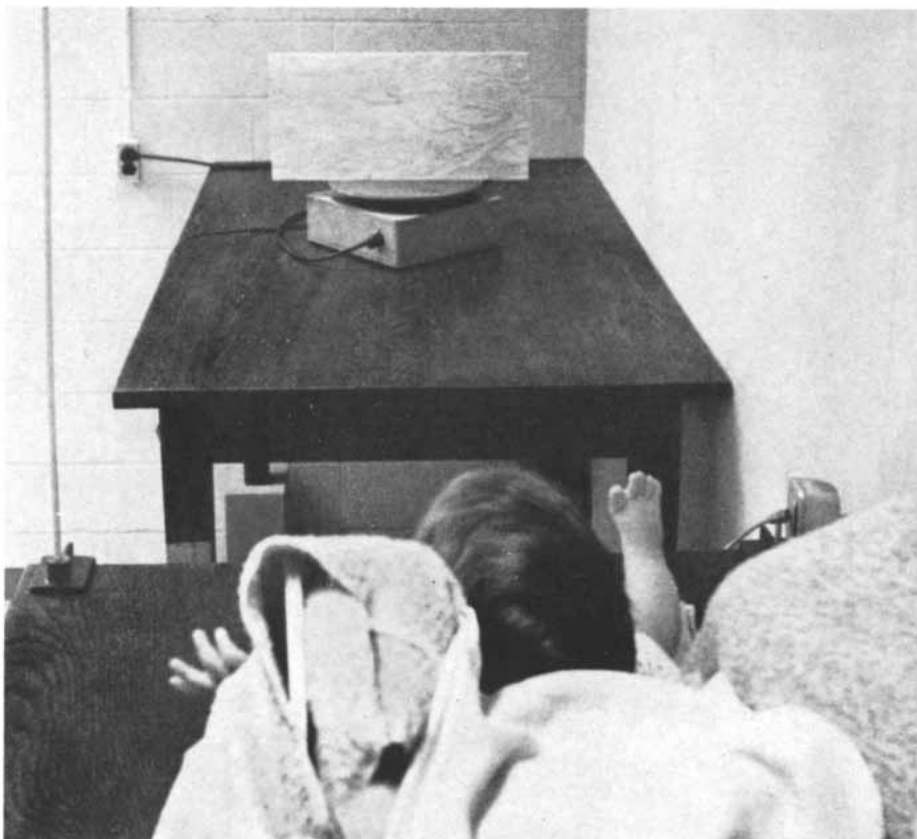
OPERANT-CONDITIONING technique requires that an infant be trained to respond to the presentation of a certain stimulus. In this experiment in shape perception the stimuli are plywood rectangles and trapezoids placed at various angles to the infant's line of sight. The object is to see how well the infant can differentiate among the shapes and orientations.
