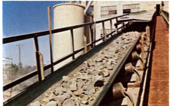
Single-ply conveyor belting is now tougher than ever. A new bi-constituent fiber used by Uniroyal combines the strength of nylon with the stability of polyester.
