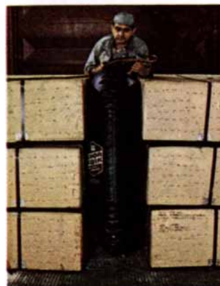
(Left.) Collapsible container is inflated to keep cargo from moving during shipment. (Right.) After run it can be deflated quickly to allow for unloading.
