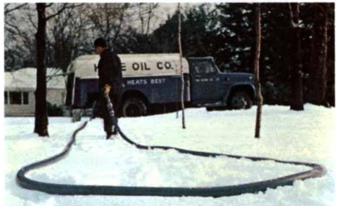
Oil hose is made of a blend of nitrile rubber and polyvinyl chloride plastic. This blend combines superior oil resistance and outstanding weathering ability.
