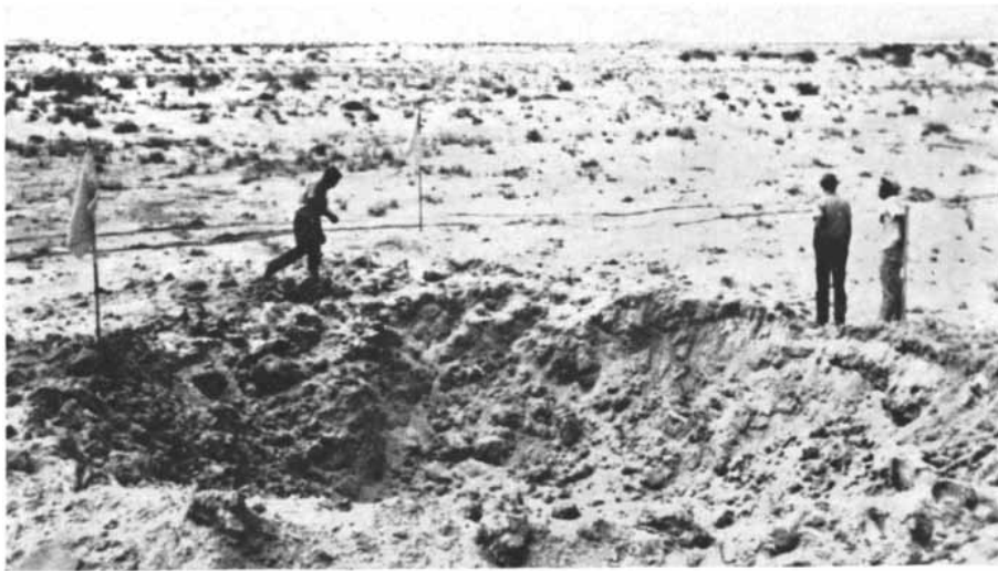
ROCKET CRATER at White Sands Proving Ground shows how rocklike lumps (instant rocks) are produced when a high-speed projectile lands in unconsolidated sandy soil.
