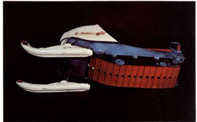
Snowmobile is an unusual application of the "tooth" principal of timing belts. Here it is used as the track belt (shown in red) to propel the vehicle.
