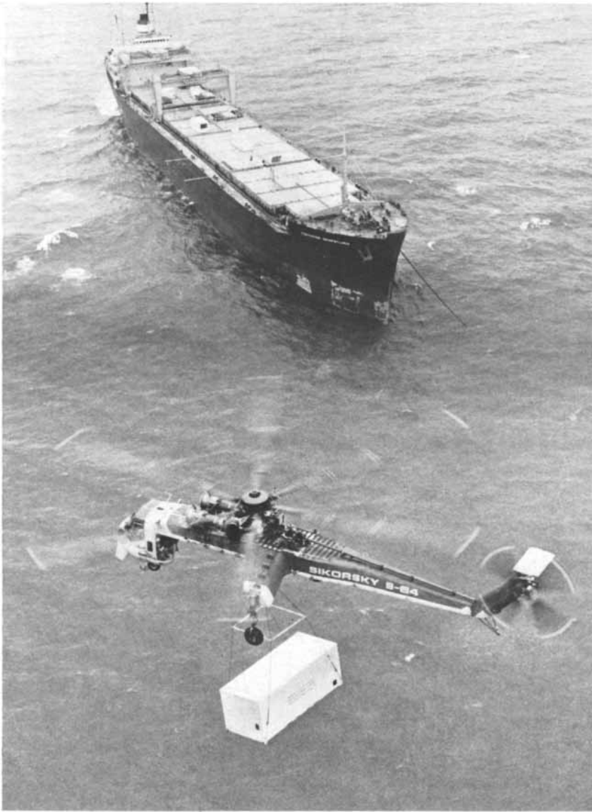
HEAVY LOADS can be handled in difficult locations by helicopters. This Sikorsky S-64 Skycrane is carrying a cargo container from a container ship to the shore. In some crowded or badly equipped harbors this could constitute an economic method of unloading a ship.
