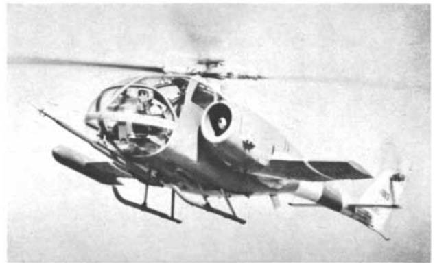
XH-51A "compound" helicopter has a hingeless rotor for maneuverability. With a jet engine and stub wings to relieve the rotor of some propulsion and lift functions, it has flown 272 miles per hour.
