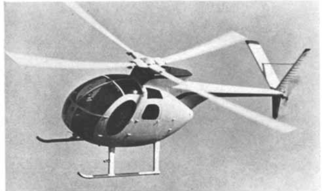
It has a two-blade teetering rotor. The Hughes 500 ( right ) has a range up to 500 miles. Both helicopters are powered by gas turbines.
