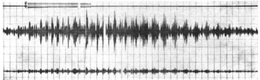
FIG. 1. Segment of micropulsation record showing high- and low-sensitivity traces. Recorded at 25 inches per hour at Honeywell's Cedar Creek Station.
