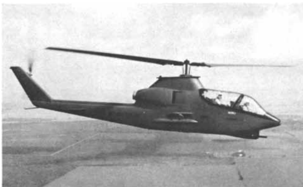
NEW MODELS are built for increased speed. The Bell "Hueycobra" ( left ), a military model, is aerodynamically clean and has retractable landing gear and stub wings for speed. The Lockheed
