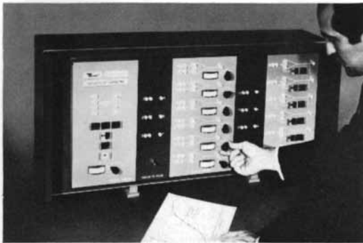
Giving machines the ability to learn. This Bendix Neurotron device, designed for the Bionics Branch of the Air Force, can be trained to perform certain recognition or control functions. Someday, similar machines may forecast weather, control spacecraft or read mail.
