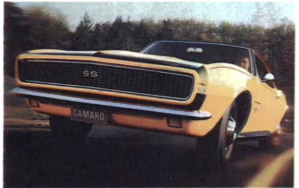
The grille of the Chevrolet Camaro is made of ABS. Because it is lightweight and tough, ABS parts are being designed for other external automotive uses.
