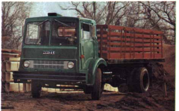
The cab of the Trend, a new truck from White Motor, is made of impact-resistant expanded ABS. It can't corrode and road noises are drastically reduced.
