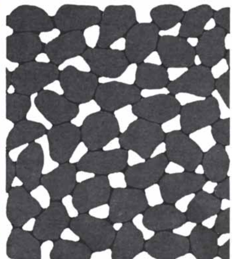
WELL-CONSOLIDATED ROCKS , in which individual grains are held together strongly, retain their structure even if fluid or gas is removed and give rise to little or no subsidence.
