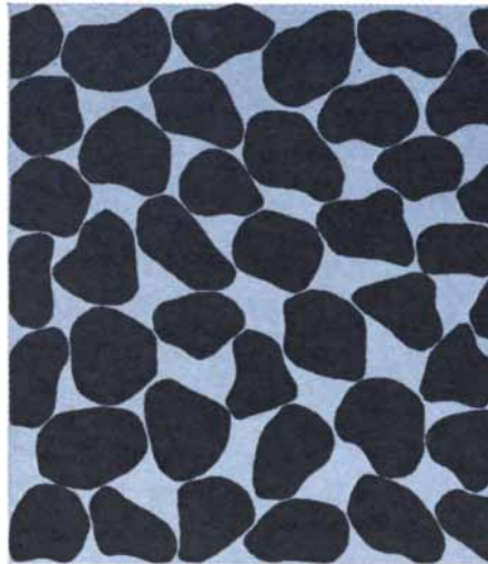
POORLY CONSOLIDATED ROCKS also can lead to subsidence when fluid is withdrawn, although the subsidence will be less because the rock is stronger than clay. In such rock the individual grains are weakly held together and will be compressed by additional pressure.
