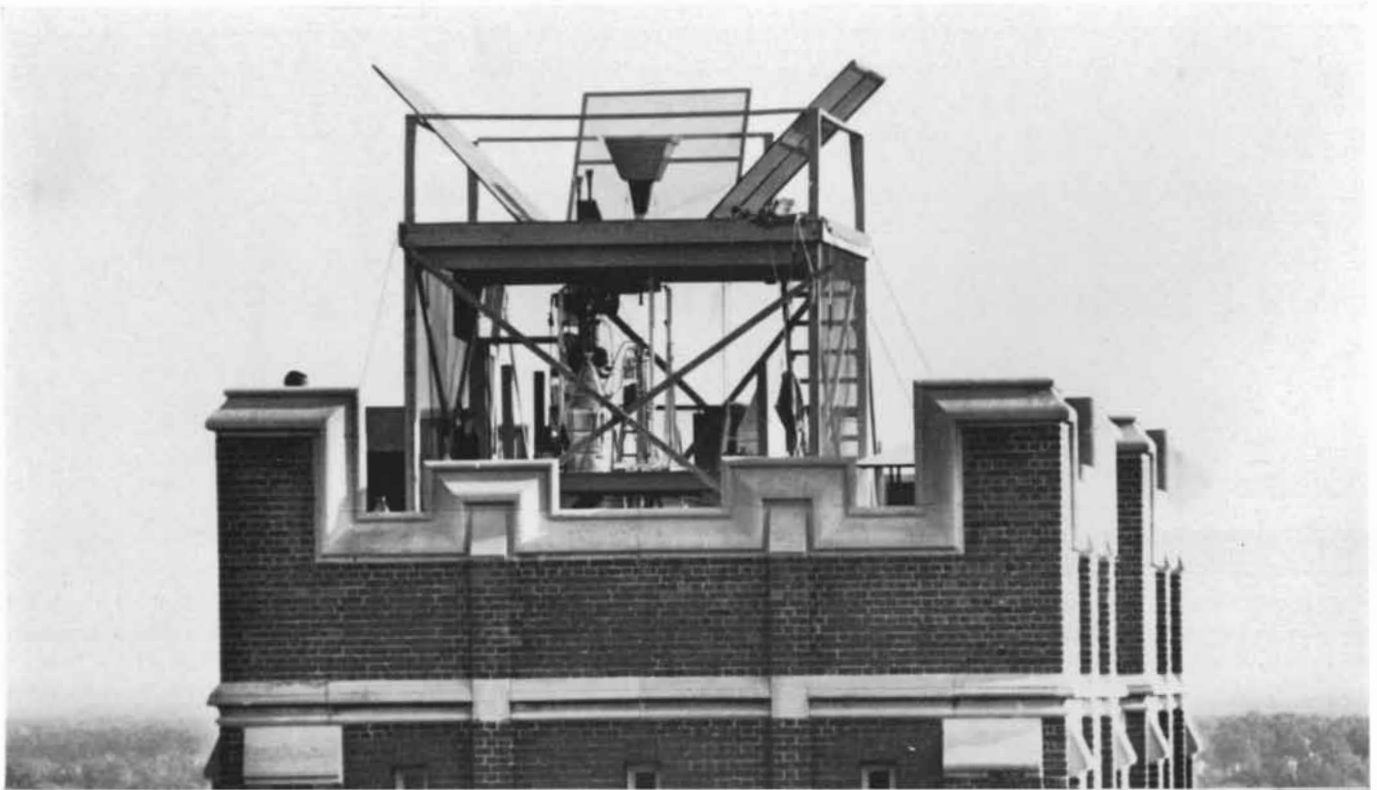
PRINCETON GROUP'S first fireball observations were made with an earlier version of the radiometer, here shown in position on the
