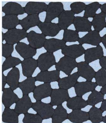
WELL-CONSOLIDATED ROCKS , in which individual grains are held together strongly, retain their structure even if fluid or gas is removed and give rise to little or no subsidence.
