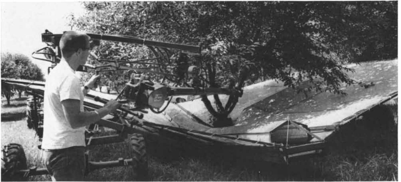
CHERRY PICKER , part of which is shown on the cover of this issue, has two arms that grip limbs of the cherry tree and shake them.
