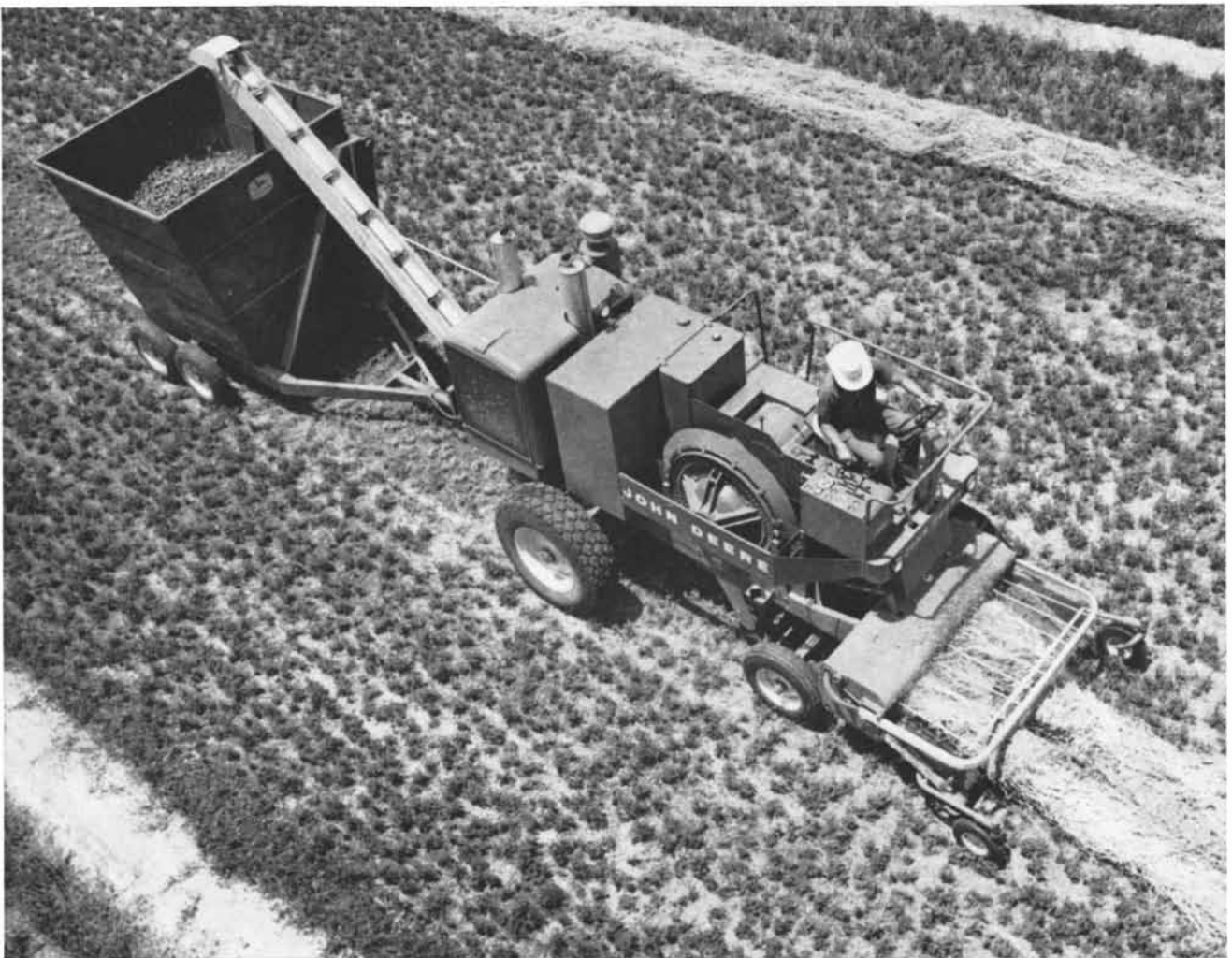
HAY-CUBER was designed to reduce the bulk of hay. It picks hay up from a windrow and compresses it into cubes of a size that cattle can eat readily. The machine was designed for alfalfa and other leg-
