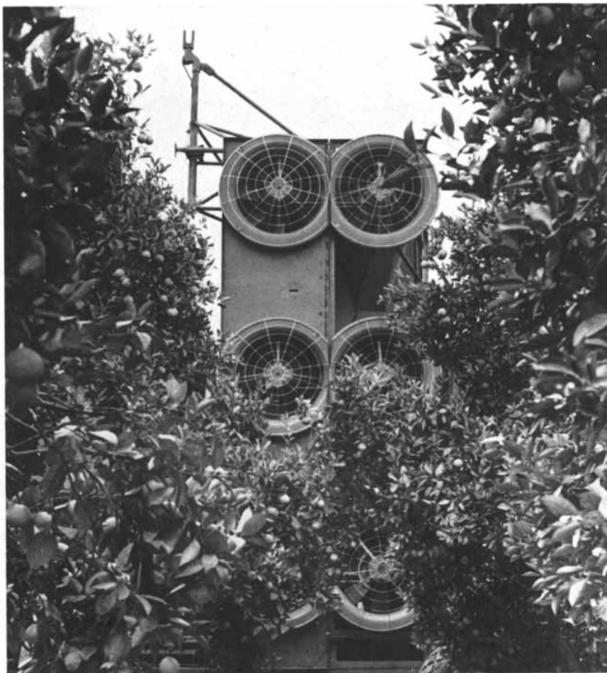
EXPERIMENTAL CITRUS HARVESTER shakes the limbs of the fruit trees with blasts of air. The fruit drops to a catching frame attached to the harvester. The machine, which was developed by the Florida Manufacturing Corporation, clears a tree in two to three minutes.
