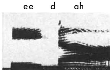
Comparison of nonsense word "eedah," pronounced by a human (left) and by Coker's program. These speech spectrographic patterns represent time (horizontal scale), frequency (vertical), and intensity (line density). The dark bars are called "formants" and are characteristic of speech sounds. The technique for making these diagrams was conceived and developed in the early 40's at Bell Telephone Laboratories.
