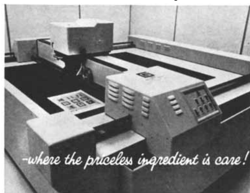
Automatic Pen Produces Intricate Final Integrated Circuit Mask
