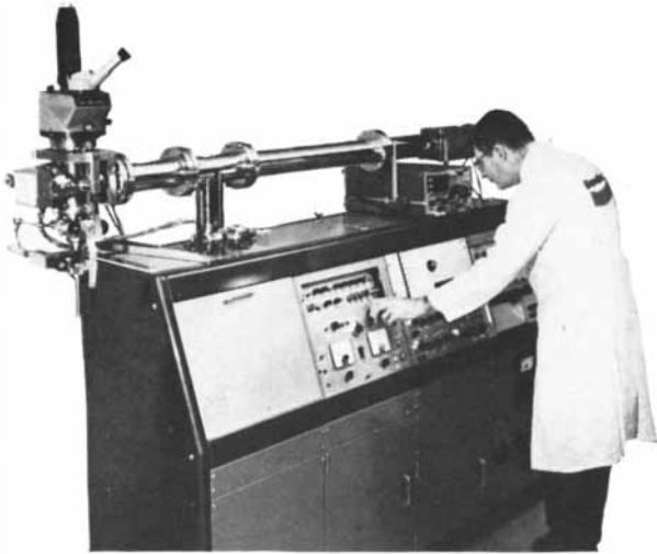
On the beam. The new Bendix Laser/TOF Microprobe Mass Spectrometer holds great promise for diagnosis of lung diseases, analysis of metal films and other analytical applications. It combines great accuracy with the energy-focusing ability of the laser.
