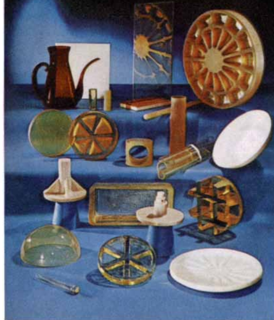
VERSATILITY of CER-VIT materials is represented by forms which are cast, pressed, blown, drawn, in flat forms, machined, transparent, translucent, opaque — and from clear to brilliant colors.
