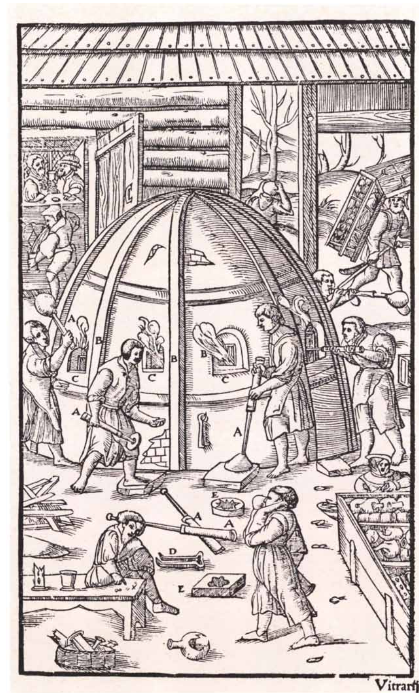
GLASS IS MADE in Georgius Agricola's De Re Metallica , published in Germany in 1556. The men around the beehive-shaped furnace are holding blowpipes for blowing the glass.
