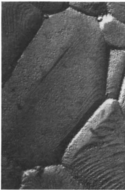
This electronmicrograph at 27,000 X shows the microstructure of new Coors AD-999 polycrystalline sapphire (alumina) ceramic, polished to a mirror finish and thermally etched to define crystal boundaries. The largest crystal is approximately 2.5 microns. An average crystal of ordinary aluminum oxide ceramic at 27,000 X magnification would be bigger than this page! You can see the secret of this new super ceramic—very fine texture, articulate crystal structure and no voids, in addition to high purity.
