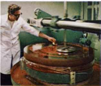
Below: Zero-expansion characteristic of CER-VIT material cuts down long waits during figuring, grinding, polishing.
