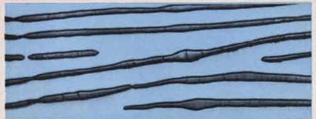
A longitudinal section of sapphire fibers in an aluminum titanate matrix. This section was produced by electron beam zone melting. The activities described here are only a few of Lockheed's current R&D projects in materials. If you are an engineer or scientist interested in this field of work, either in California or Georgia, Lockheed invites your inquiry. Write: K. R. Kiddoo, Lockheed Aircraft Corporation, Burbank, California. An equal opportunity employer.
