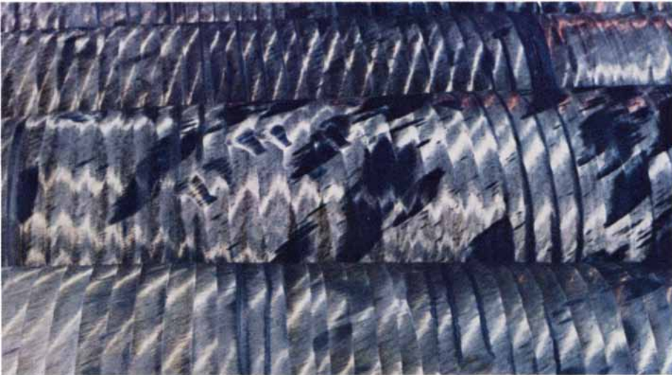
Rough-grinding high-strength Discaloy® ingots
