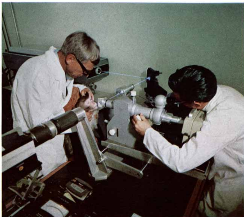
In initial tests using a rhesus monkey, two members of the research team at Stanford control the blue-green beam from a Model 140 continuous wave argon laser by means of a shutter mechanism and an optics aiming device.
