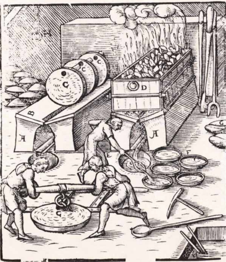
CAKES OF COPPER-LEAD ALLOY ARE HEATED to get silver from copper in a book by Lazarus Ercker published in Prague in 1574. Silver was contained in molten lead (center).
