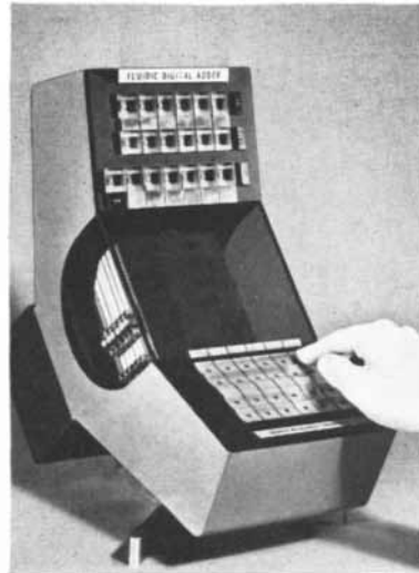
In a fluid state. Here is a digital computer that performs its functions with fluidic—instead of electronic—circuits. Bendix developments like this in the new field of fluidics might someday lead to such things as a “kitchen computer” for the home.
