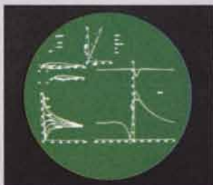
Viewer displays synthesized wing design plus performance data.
